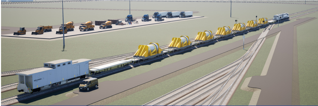
The U.S. Department of Energy's concept for a potential transport train for commercial used nuclear fuel.
