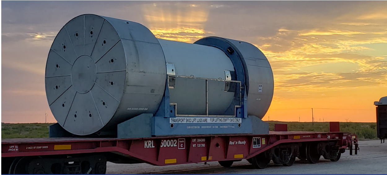
A Type B cask for transporting radioactive material on a railcar. Photo credit: Orano.
