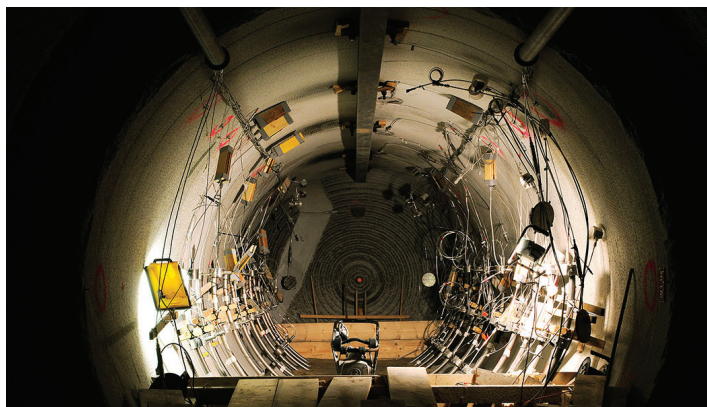
Grimsel Test Site (Switzerland): Gas Permeable Seal Test Experiment – In-Situ Instrumentation Prior to Seal Emplacement. Courtesy of I. Blechschmidt (Swiss National Cooperative for the Disposal of Radioactive Waste).
