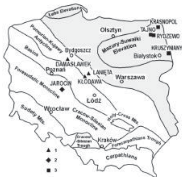
Figure 21.1. Location of candidate sites for the geological radioactive waste repository in Poland shown on a simplified geological map: (1) salt domes; (2) shale; (3) igneous rocks (granites and other)
