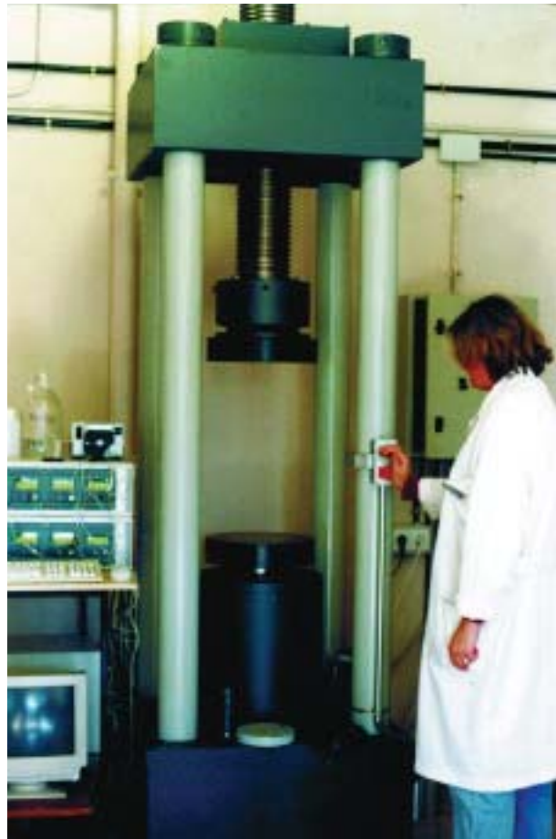
Figure 27.7. Pore-water extraction equipment
