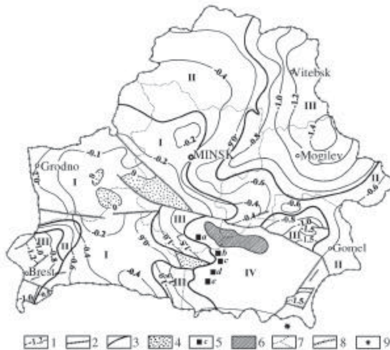
Figure 4.4. Geological division of Belarus into zones in accordance with conditions for medium- and high-level radioactive waste isolation.
