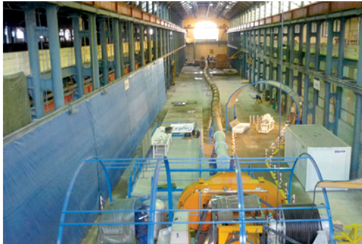
Figure 16 – Retrieval test of a HLW package from a heavily deformed cell
