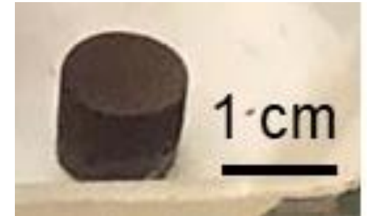
Sintered SIMFUEL pellet
