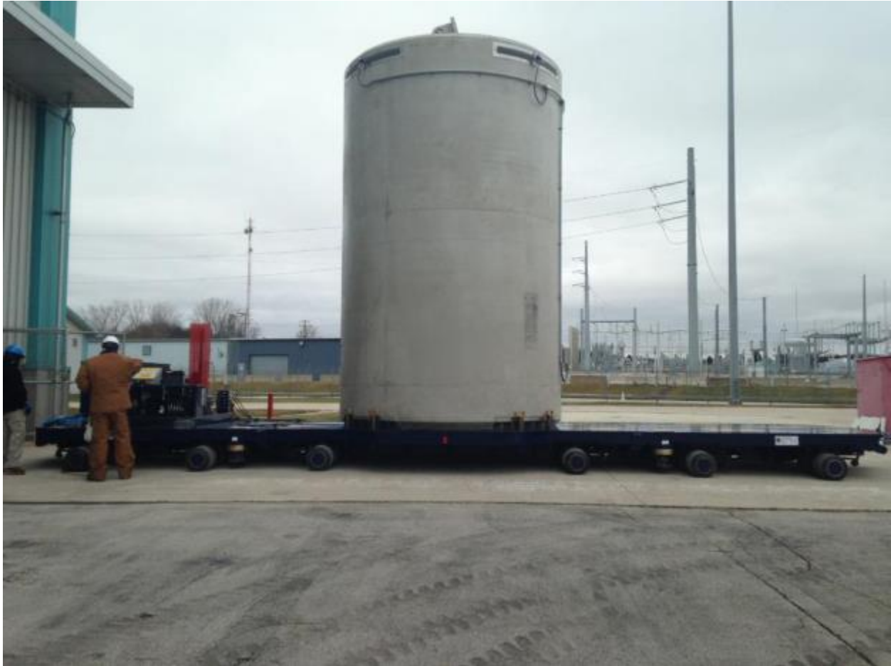
FIGURE 2-16: LOADED MAGNASTOR VERTICAL CONCRETE CASK (CC4) [19] MOVING FROM KPS FUEL BUILDING
