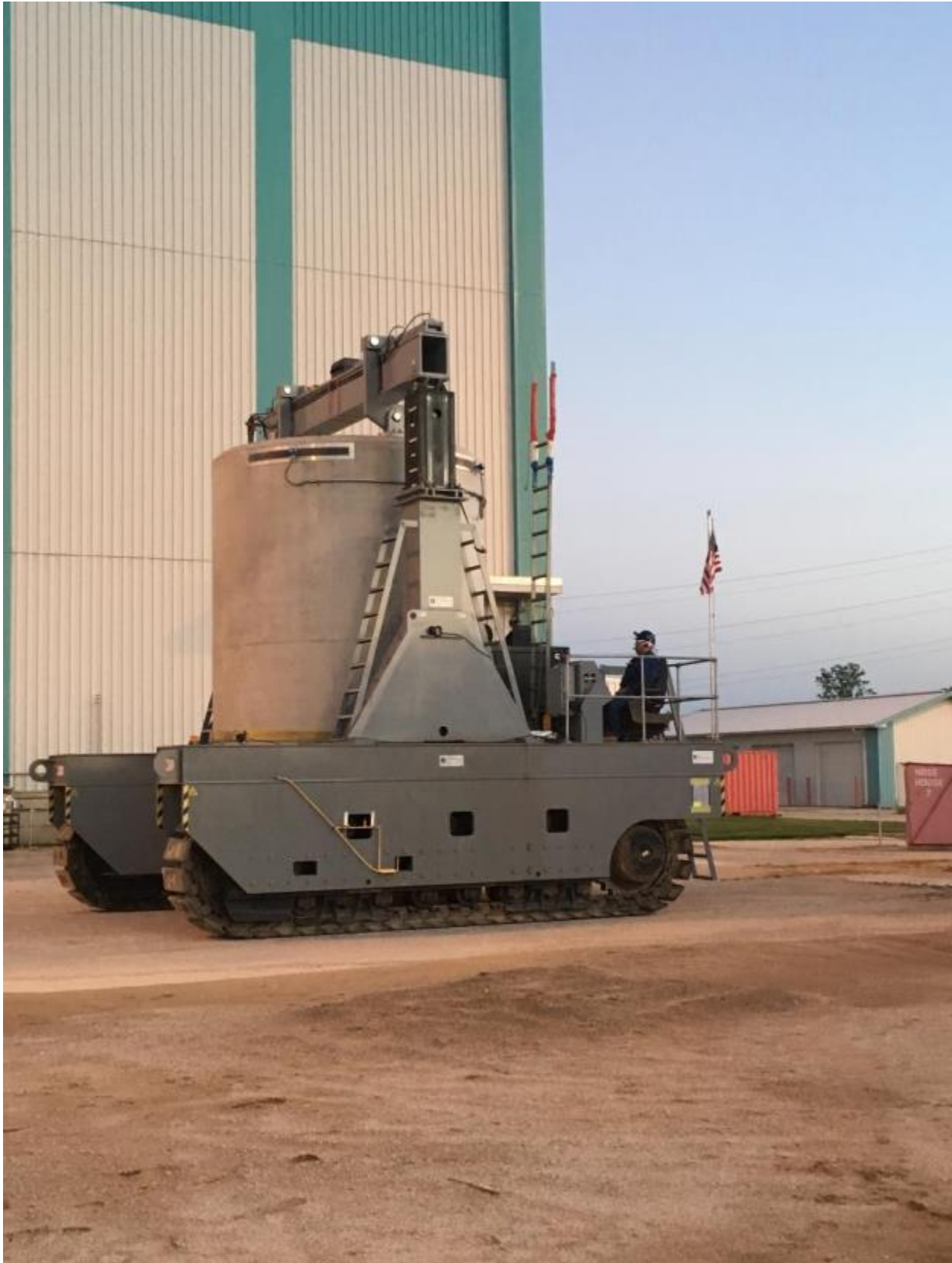
FIGURE 2-30: MAGNASTOR VCC ENGAGED TO SELF-PROPELLED VCT
