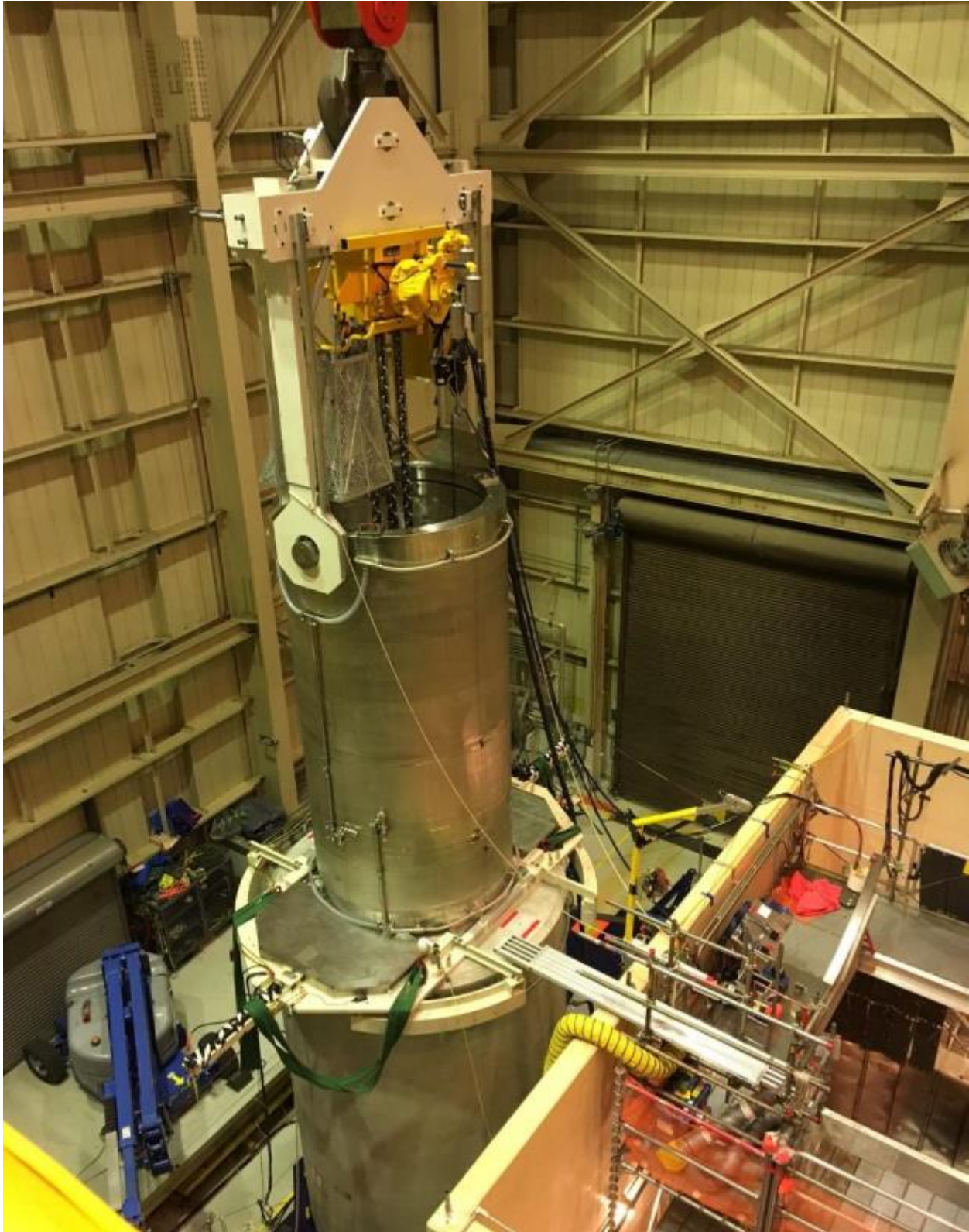
FIGURE 2-18: MAGNASTOR TRANSFER CASK (MTC2) [41] WITH TRANSFER ADAPTER ON VCC FOR TSC TRANSFER WITH SECURE-LIFT YOKE AND CHAIN HOIST
