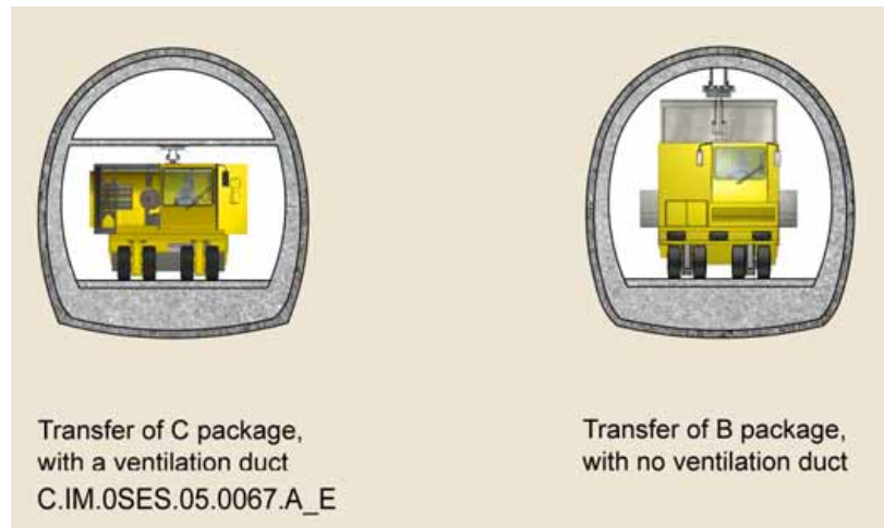
Figure 7.4.5 B and C waste package transfer drifts
