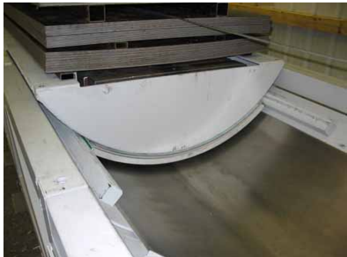
Figure 9.3.22 Tests of moving a load simulating the shape and weight of a type CUI spent fuel disposal package using air cushions
