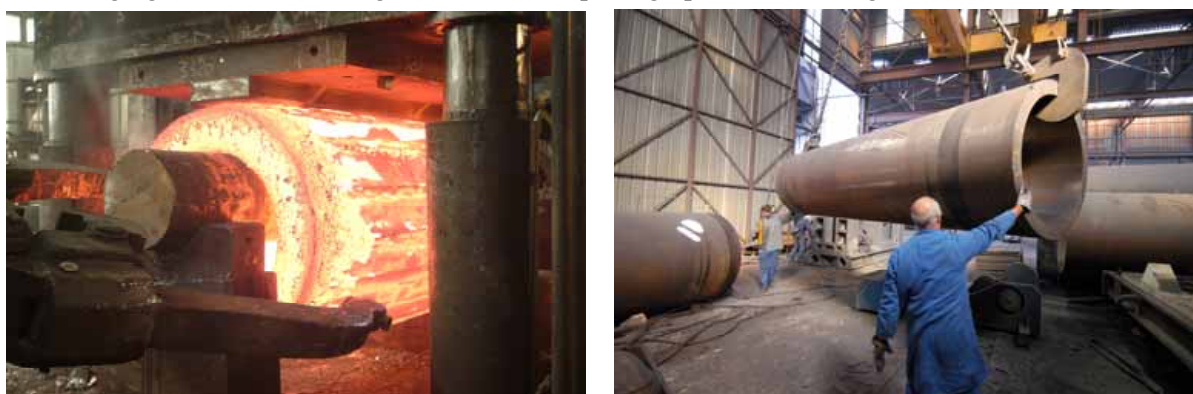
Figure 4.3.11 Manufacturing stages of shell in non-alloy steel
