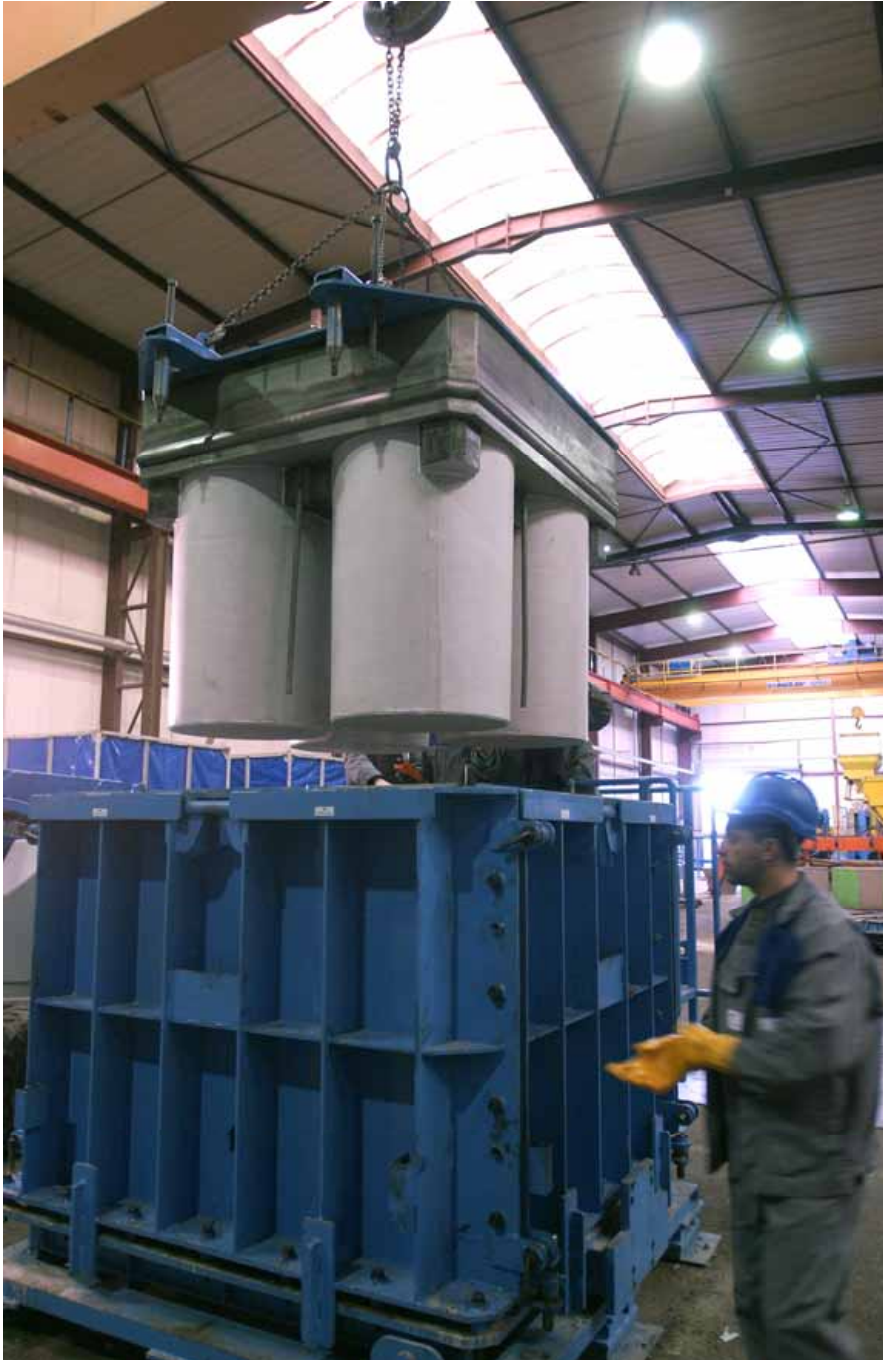
Figure 4.1.8 Installation of cores in the standard B2 package mould before casting
