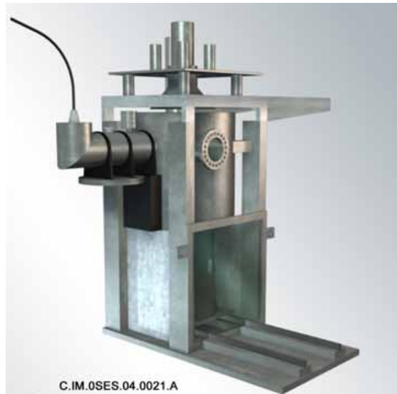
Figure 4.2.11 Welding enclosure under vacuum conditions
