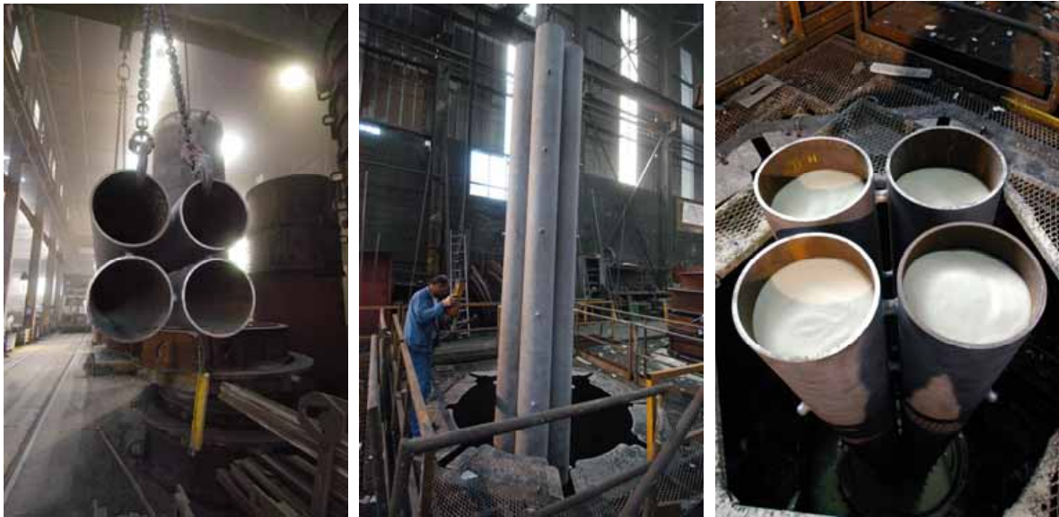
Figure 4.3.12 Preparation for insert casting
