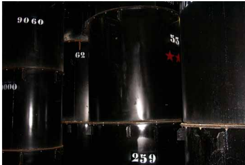
Figure 3.2.7 Non-alloy steel container used as overdrum for 1800-litre concrete containers
