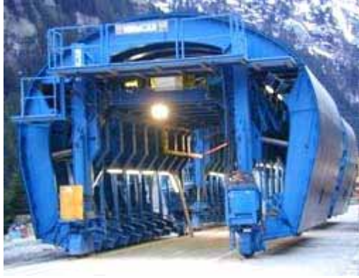
Figure 5.1.24 Mobile formwork for tunnel
