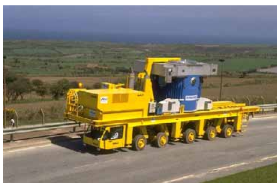
Figure 9.2.8 The transfer vehicle used on the La Hague site (doc from Cogema)
