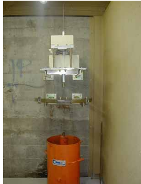
Figure 10.3.2 Measuring table for a vertical pendulum
