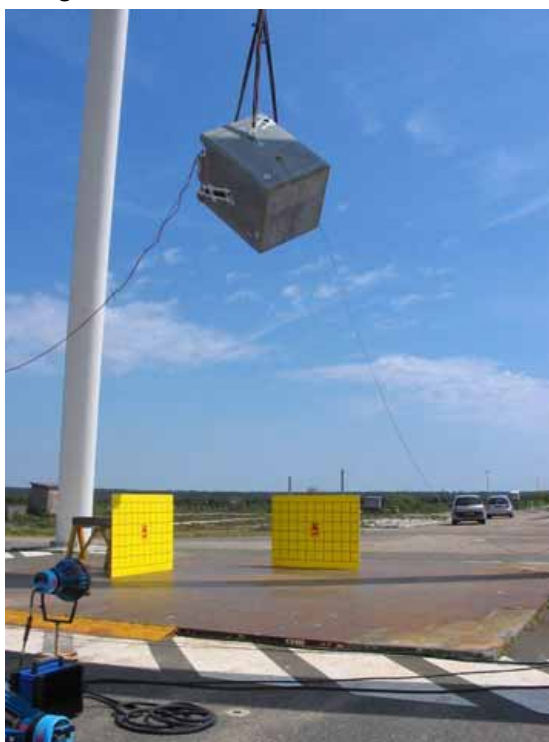
Figure 11.8.1 Installation of the drop-test demonstrator (package B5.2 - CEA/CESTA Test Centre - Gironde)
