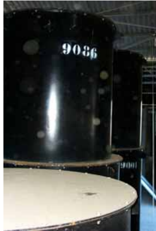
Figure 3.2.5 Non-alloy steel container used as overdrum for 1000-litre concrete containers
