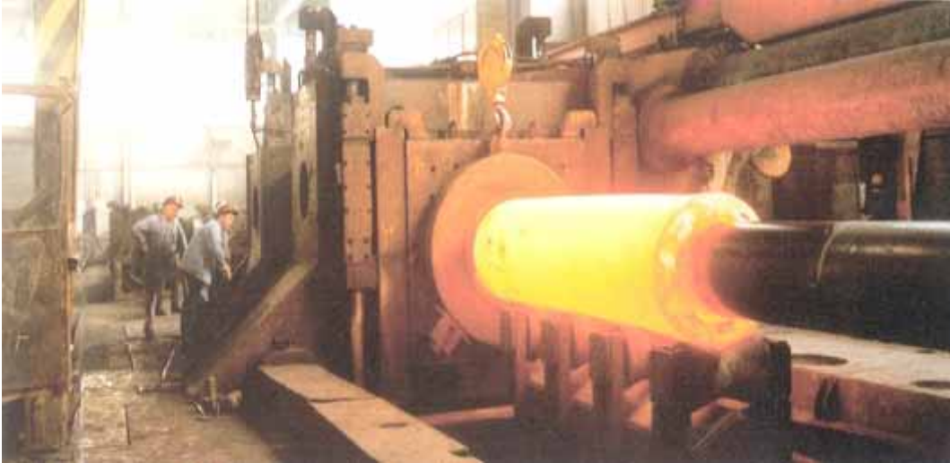
Figure 4.2.7 Drawing in an extrusion die using a mandrel and a horizontal press
