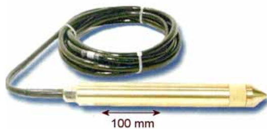
Figure 10.3.4 Vibrating wire interstitial pressure cells
