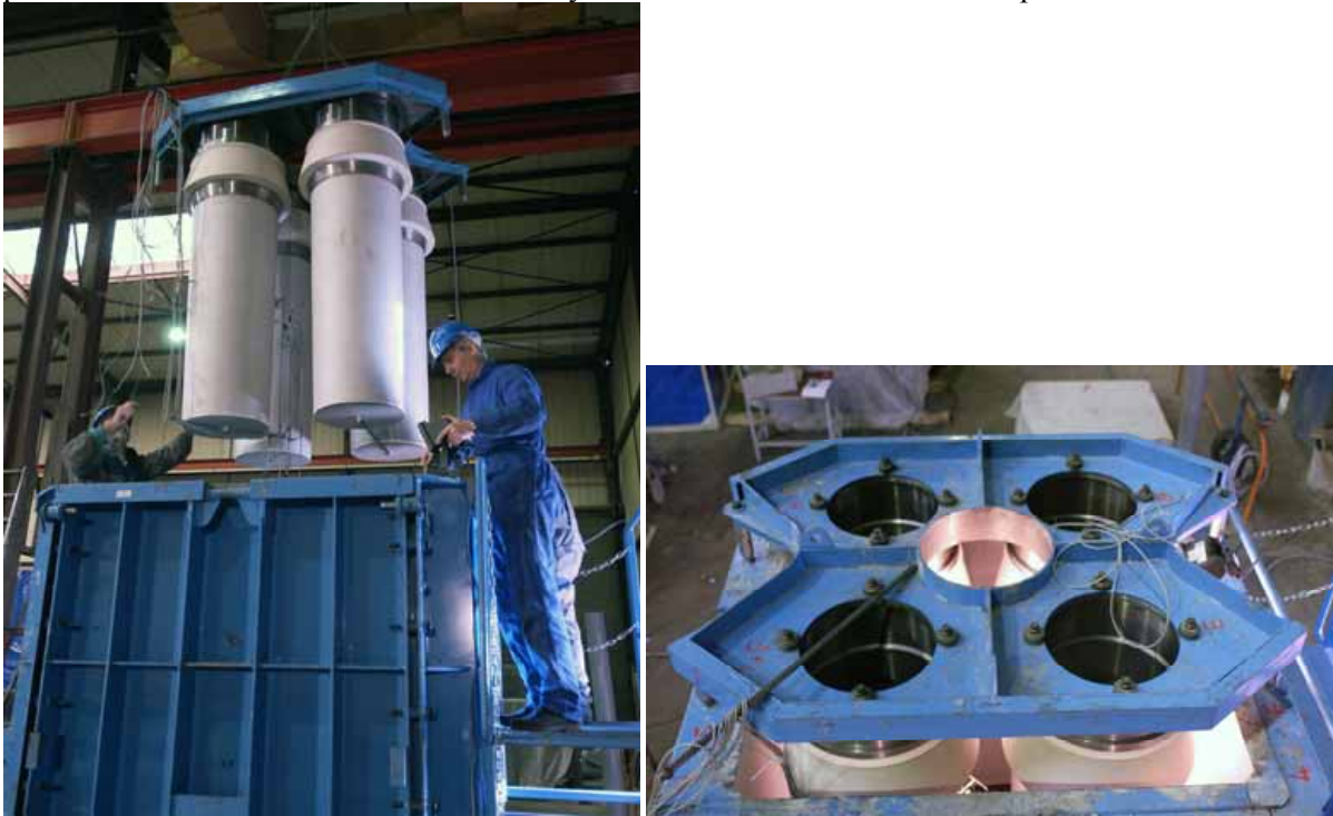
Figure 4.1.10 Installation of cores in the standard B5 package mould before casting
