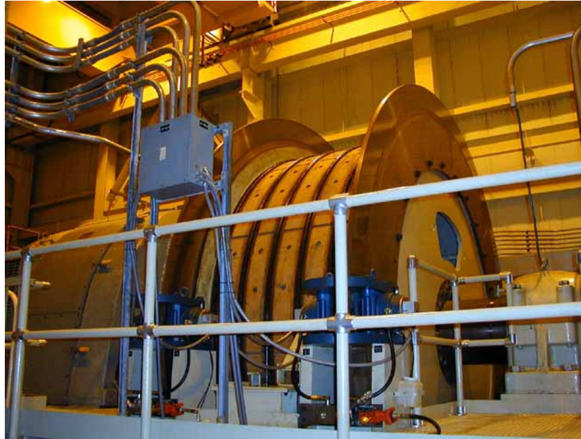
Figure 9.2.5 Koepe pulley of the WIPP packages descent shaft (USA)
