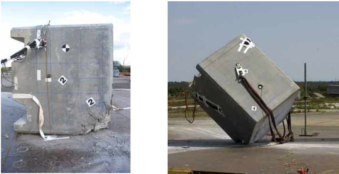
Figure 11.8.2 Appearance of the demonstration model after the drop (left, demonstration model B2.1; right, demonstration model B5.2)
