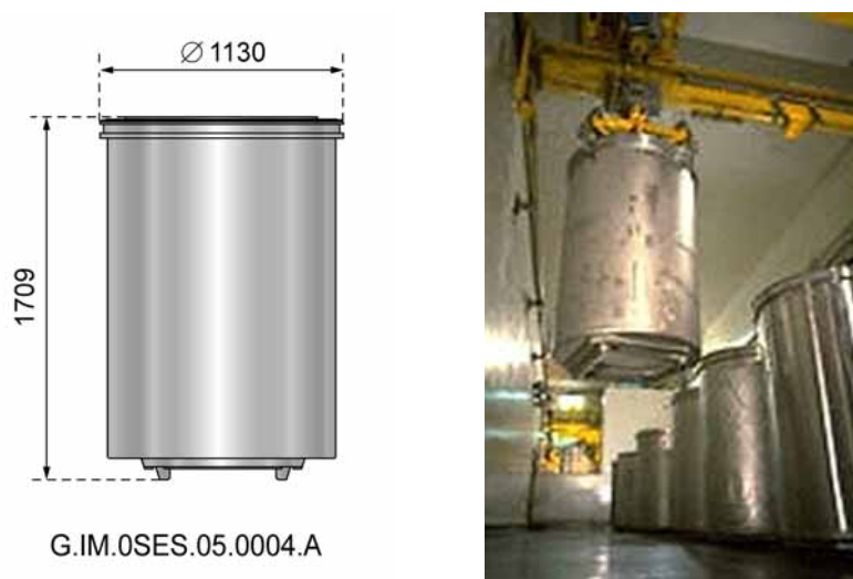
Figure 3.2.13 1,800-litre, stainless steel drum containing cemented cladding waste.
