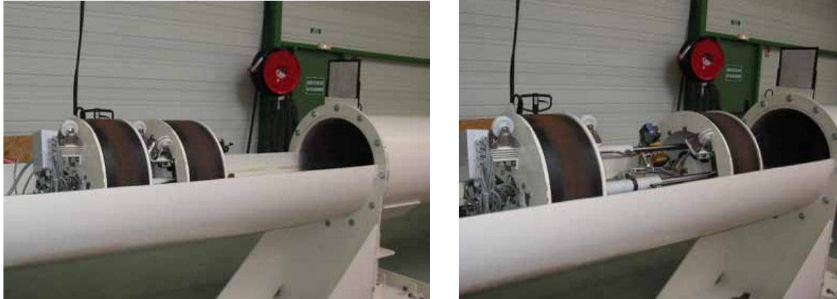
Figure 9.3.15 Pusher robot in retracted position (left) and in the deployed position (right)
