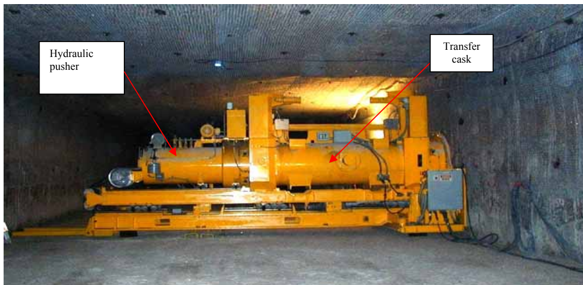
Figure 9.3.16 Transfer cask equipped with a hydraulic pusher for installing type RH wastes in horizontal cells at the WIPP disposal facility.
