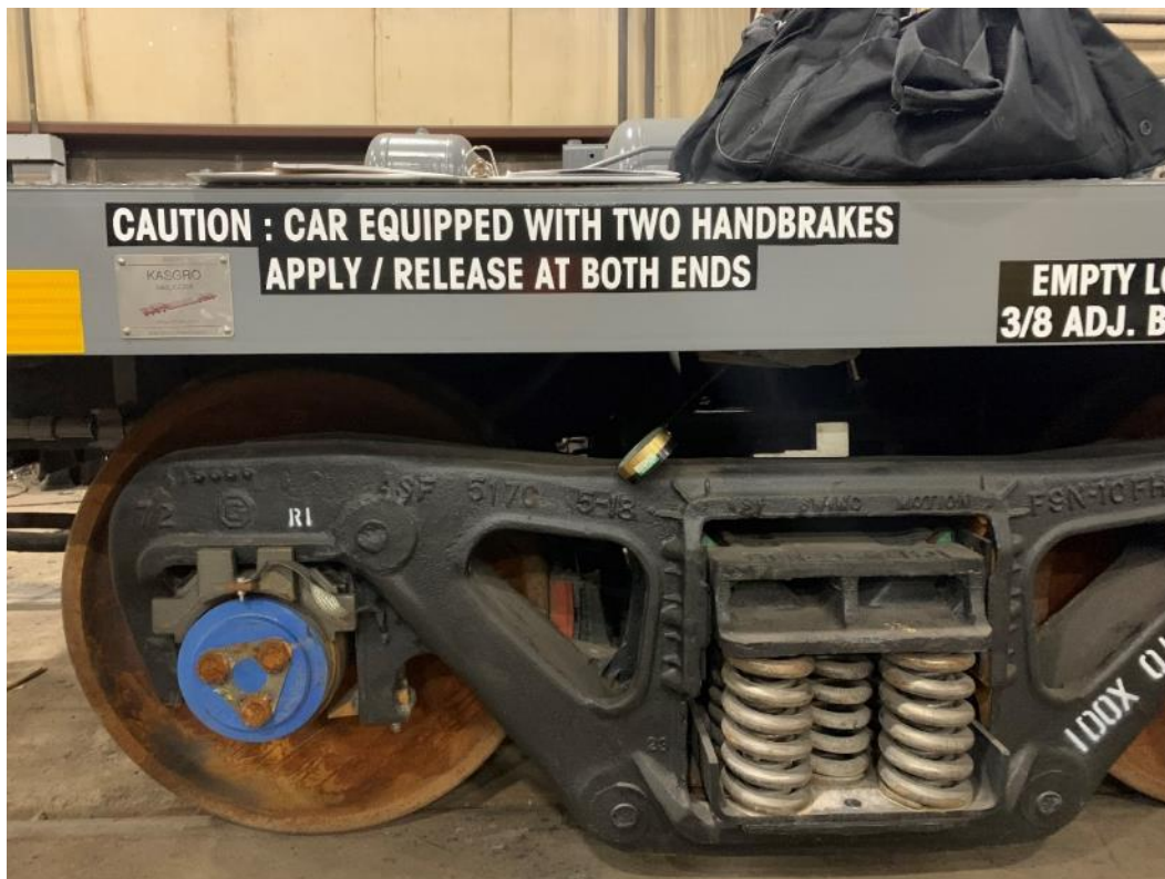
Figure C9. Brake Cylinder Pressure Gauge and Empty/Load Device
