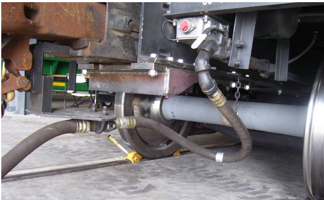
Figure 50. Coupler Carrier Plate after the Coupler Vertical Load Test
