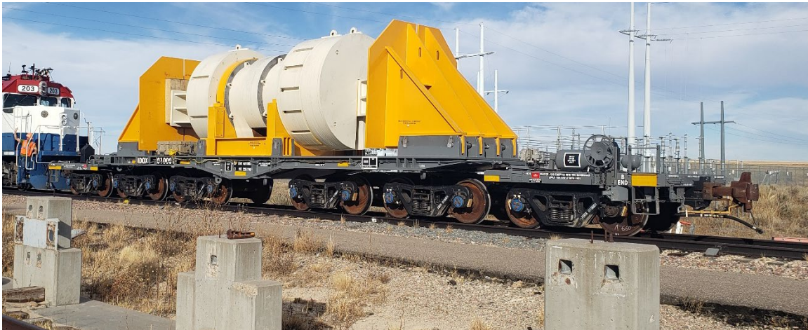
Figure 7. Maximum Test Load Assembly with End Stops Mounted on Atlas Railcar
