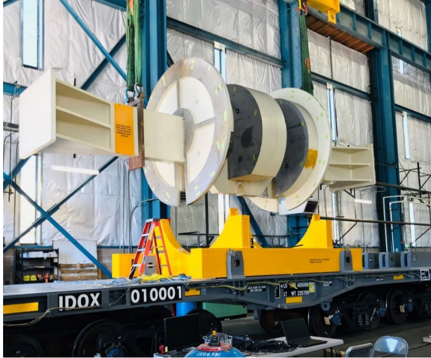
Figure 5. Central Beam Assembly Being Mounted on Minimum Test Load Cradle
