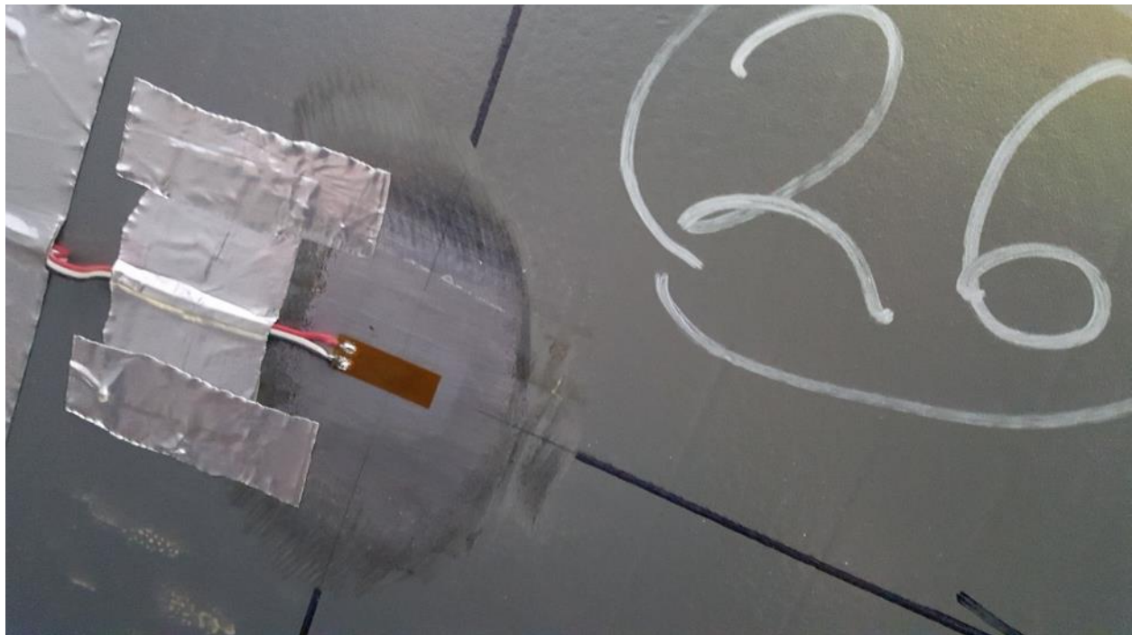
Figure D30. SGBF26 Center of LH Side Sill Bottom Flange, approximately 2" aft of #2 Cross Bearer
