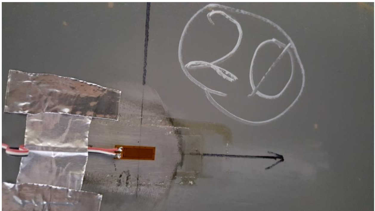
Figure D24. SGBF20 Center Sill Bottom Flange, aligned with RH Center Sill Web, at Longitudinal center of Car
