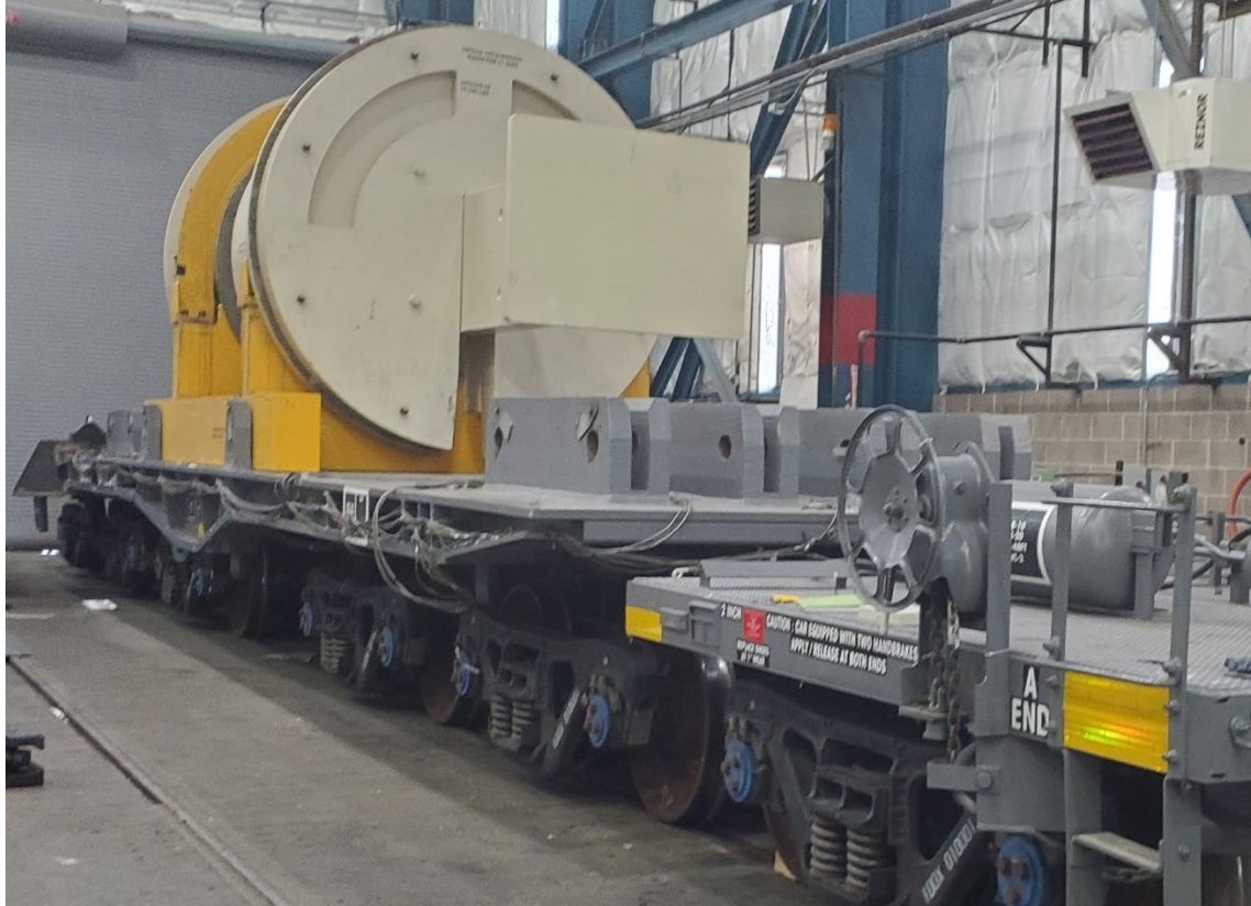
Figure 66. Cask installation in securement mounts
