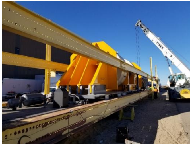
Figure F1. Atlas Car set-up in Squeeze Frame
