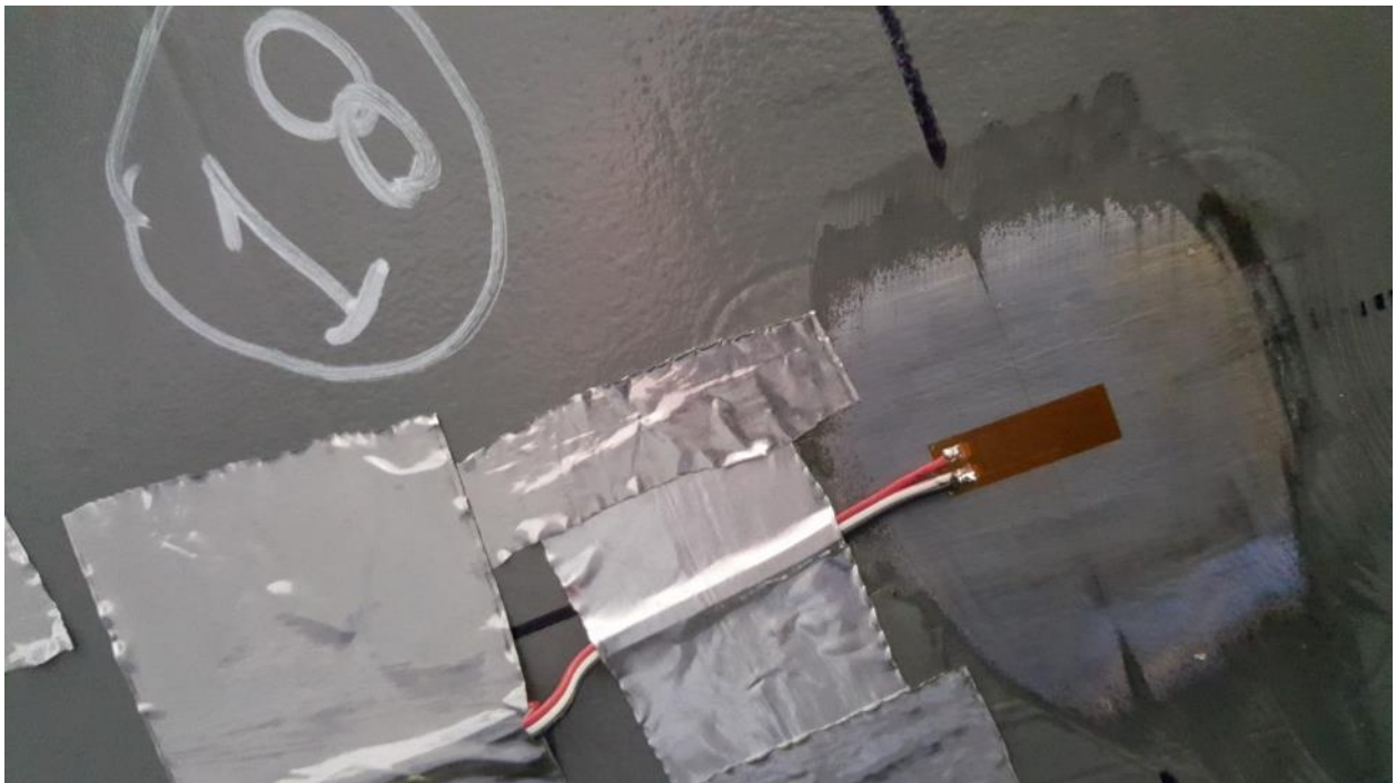
Figure D22. SGBF18 Center of LH Side Sill Bottom Flange, approximately 2" forward of #3 Cross Bearer
