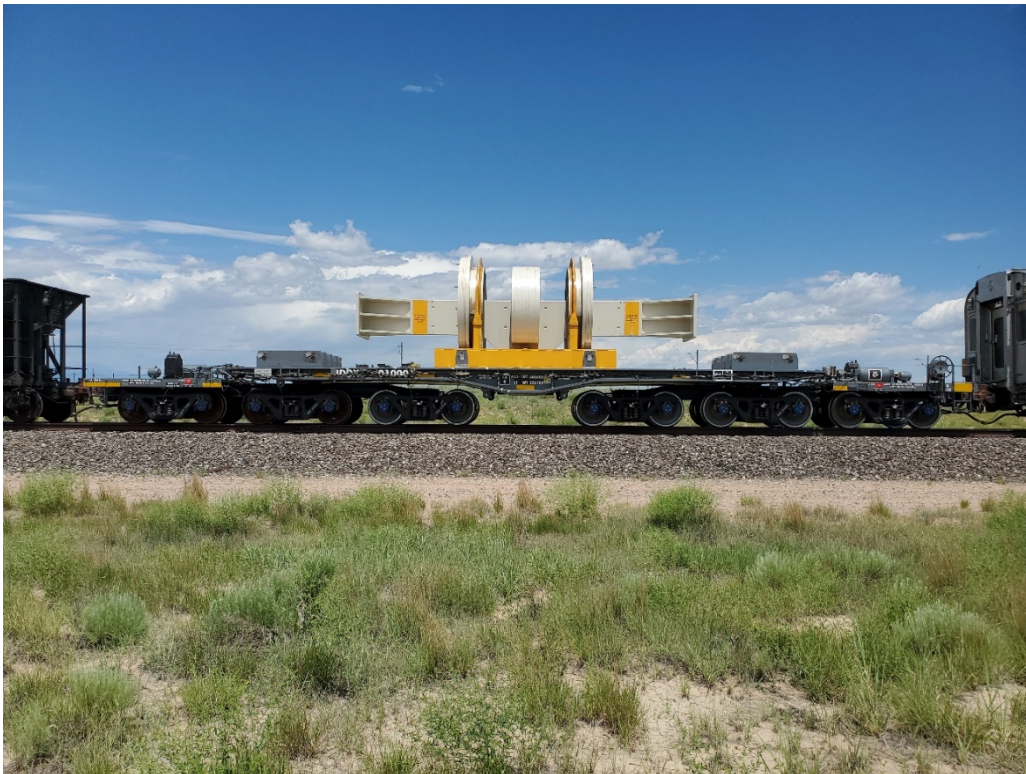
Figure 6. Minimum Test Load Assembly Mounted on Atlas Railcar
