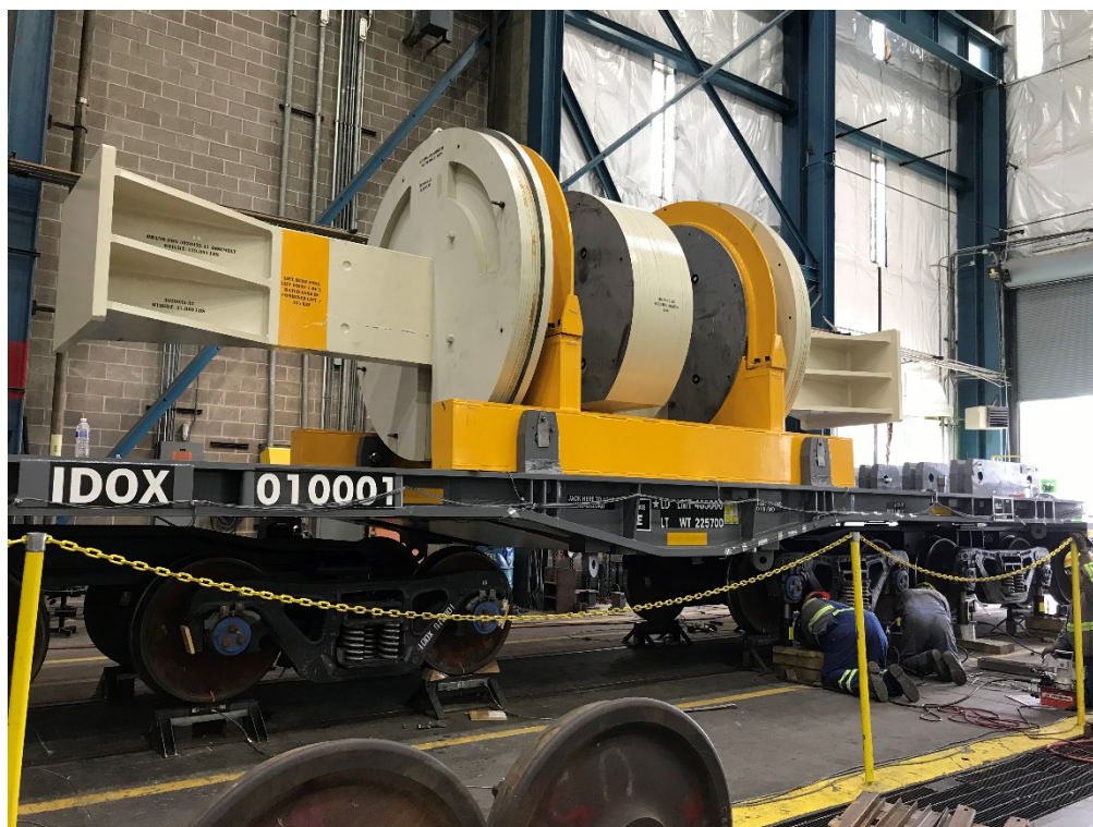
Figure 37. Atlas Railcar with Minimum Test Load during Carbody Twist Equalization Test
