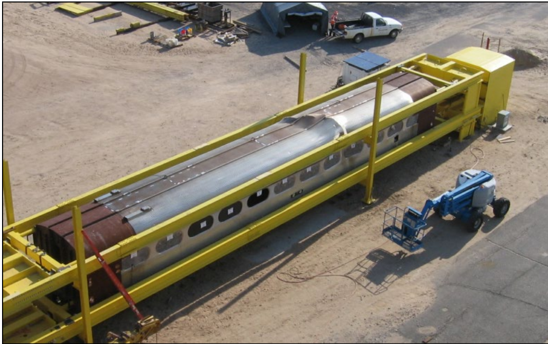
Figure 14. 2 1/2 Million Pound Squeeze Test Fixture with Passenger Car Taken to Structural Failure
