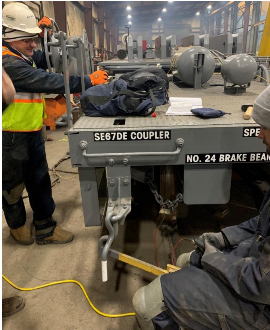
Figure C20. Smart Hook Force Measurement Device
