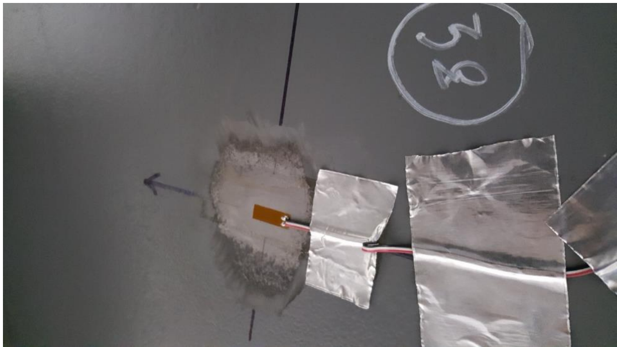
Figure D42. SGBF38 Front of Bottom Flange of Front Body Bolster near Center Sill, LH Side
