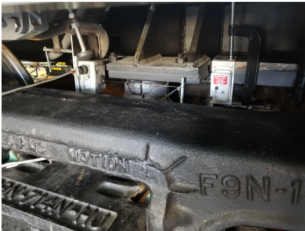
Figure 25. String Potentiometers Used for Truck Rotation Measurement
