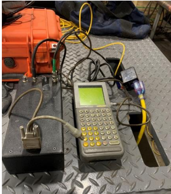
Figure C16. Jim Shoe II Brake Force Measurement System
