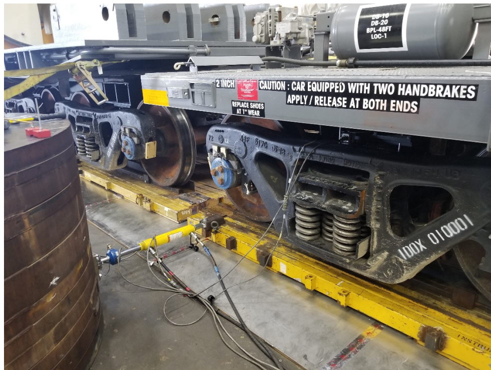
Figure 23. Truck Rotation Setup with Truck Floating on Air Table and One Lateral Actuator
