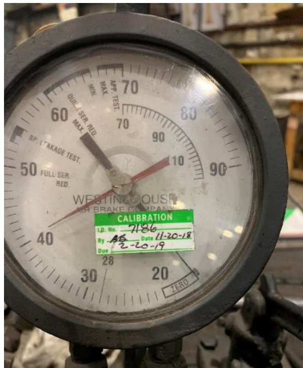
Figure C8. Single Car Air Brake Test Device Calibration Information
