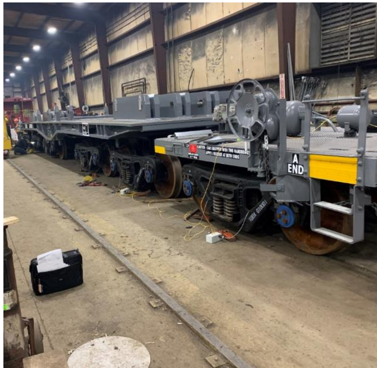
Figure C14. Three Truck Brake Shoe Force Test Setup
