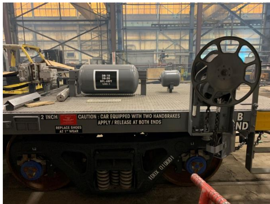
Figure C4. Cask Car B-End Brake System
