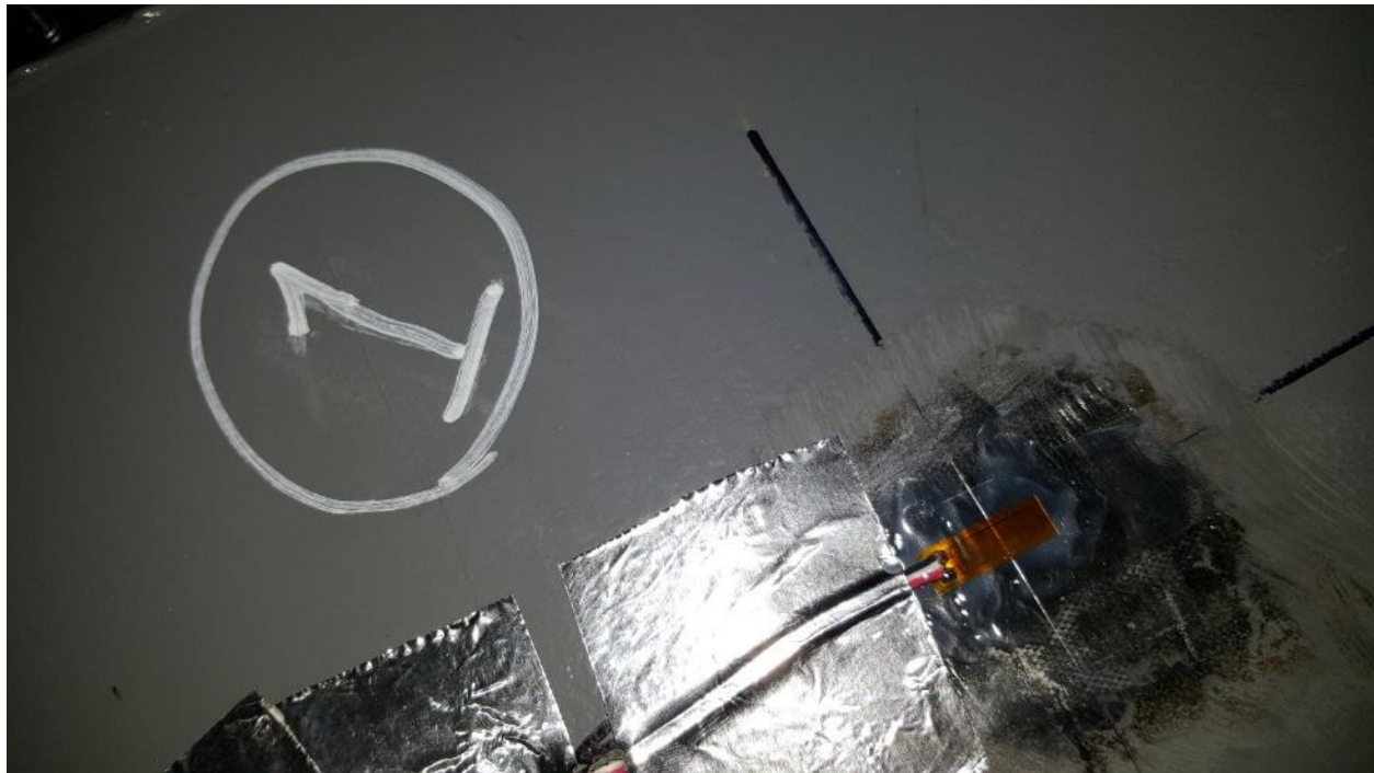
Figure D5. SGBF 1 Front of Bottom Flange of From Body Bolster near Center Sill, RH Side
