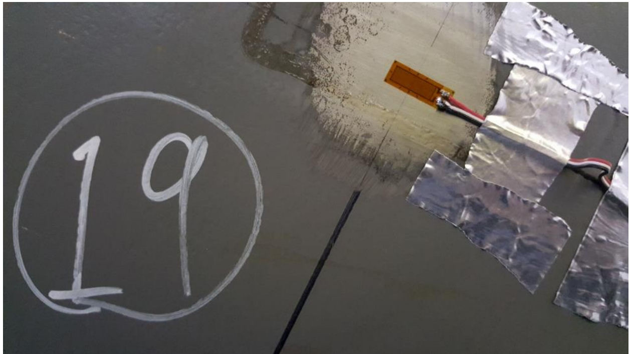
Figure D23. SGBF19 Center of RH Side Sill Bottom Flange, at Longitudinal center of Car
