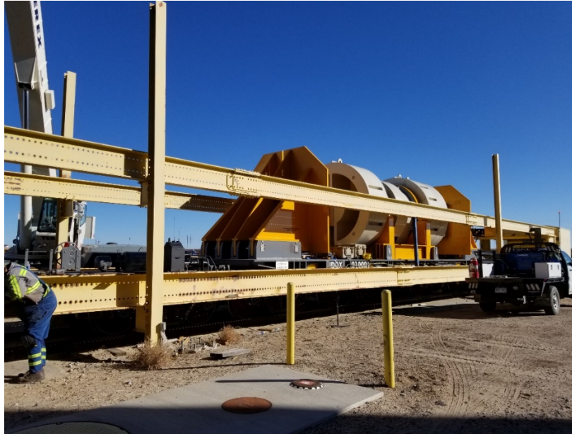
Figure 44. Maximum Test Load Compressive End Load Test
