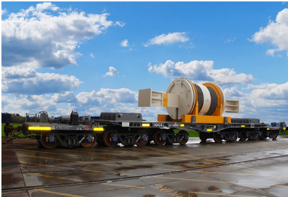
Figure 1. IDOX 010001 during Testing with Minimum Test Load
