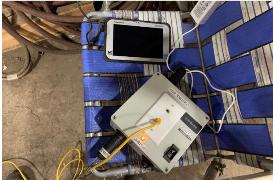
Figure C18. Pro Shoe Brake Force Measurement System
