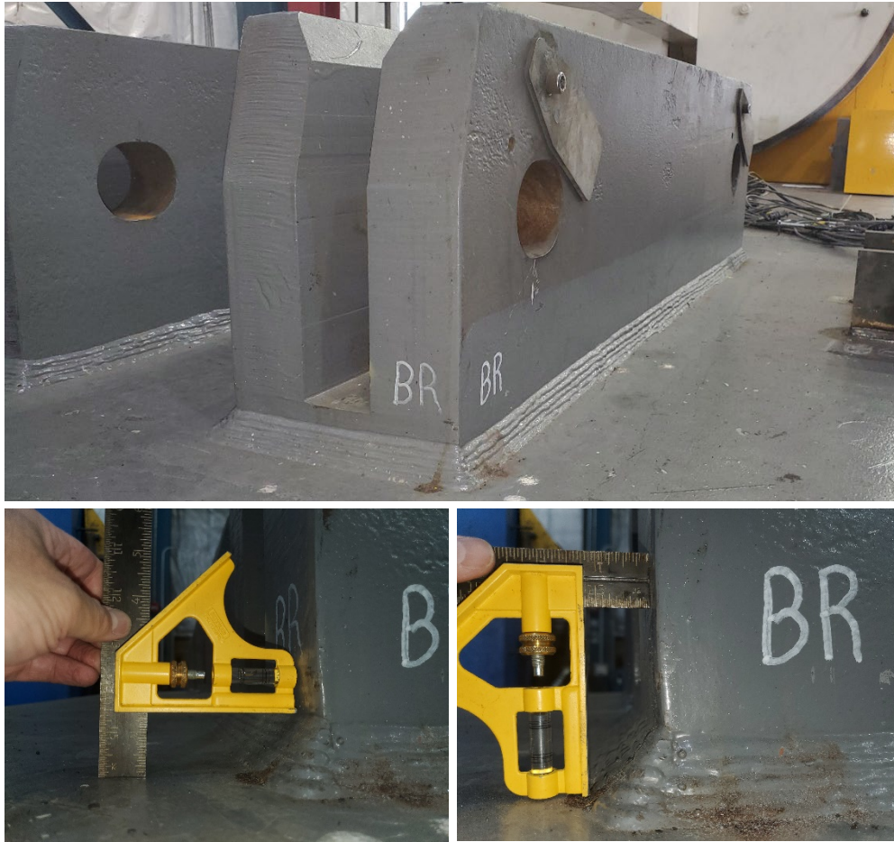
Figure 89. Example securement system welds and measurements
