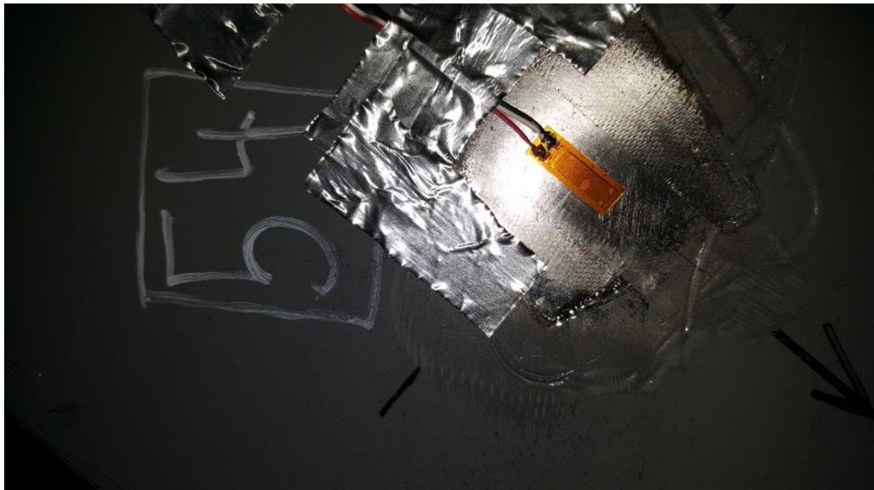
Figure D58. SGBF54 Center of Bottom Flange of Cross Bearer #3, centered in open space between LH Side Sill Bottom Flange and Center Sill Bottom Flange
