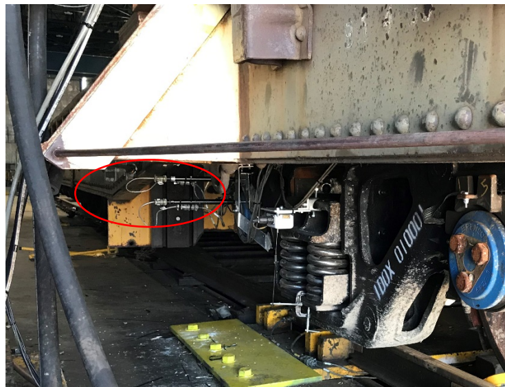
Figure 19. Instrumentation Setup to Measure Lateral Movements of Pads
