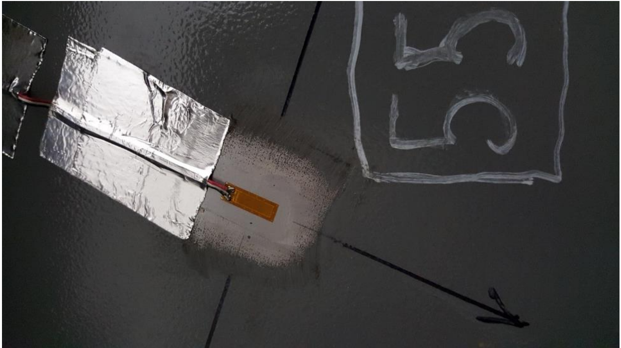
Figure D59. SGBF55 Center of Bottom Flange of Cross Bearer #2, centered in open space between LH Side Sill Bottom Flange and Center Sill Bottom Flange
