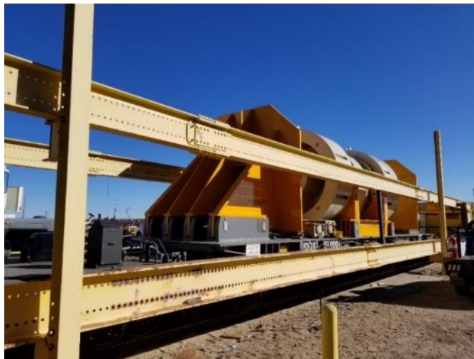
Figure F2. Atlas Car Ready for the Compression Test
