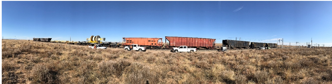
Figure 40. Atlas Railcar during the Static Curve Stability Test
