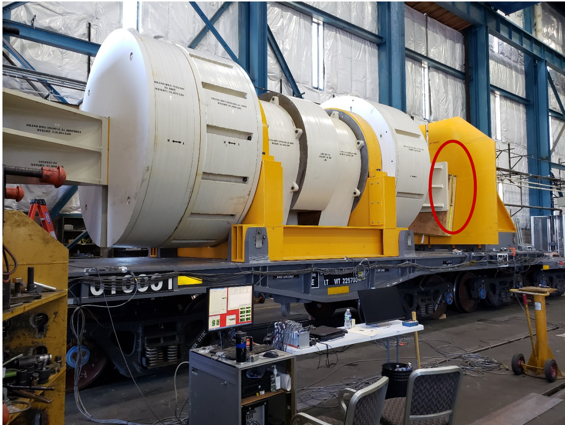
Figure 33. Atlas car with maximum test load in the RDL. Note the central beam assembly contacts the end stops.
