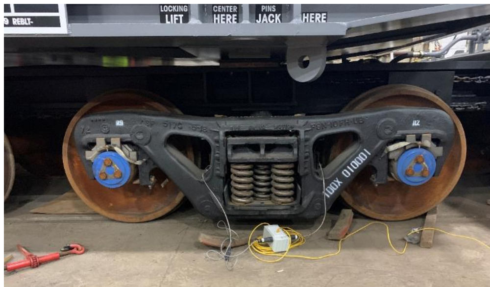
Figure C12. Example Brake Shoe Force Test Sensor Setup
