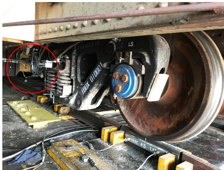
Figure 12. String Potentiometer for Measuring Spring Vertical Displacement
