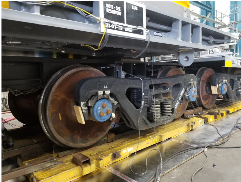
Figure 24. Test Setup for the Span Bolster Test Showing Connected Air Tables
