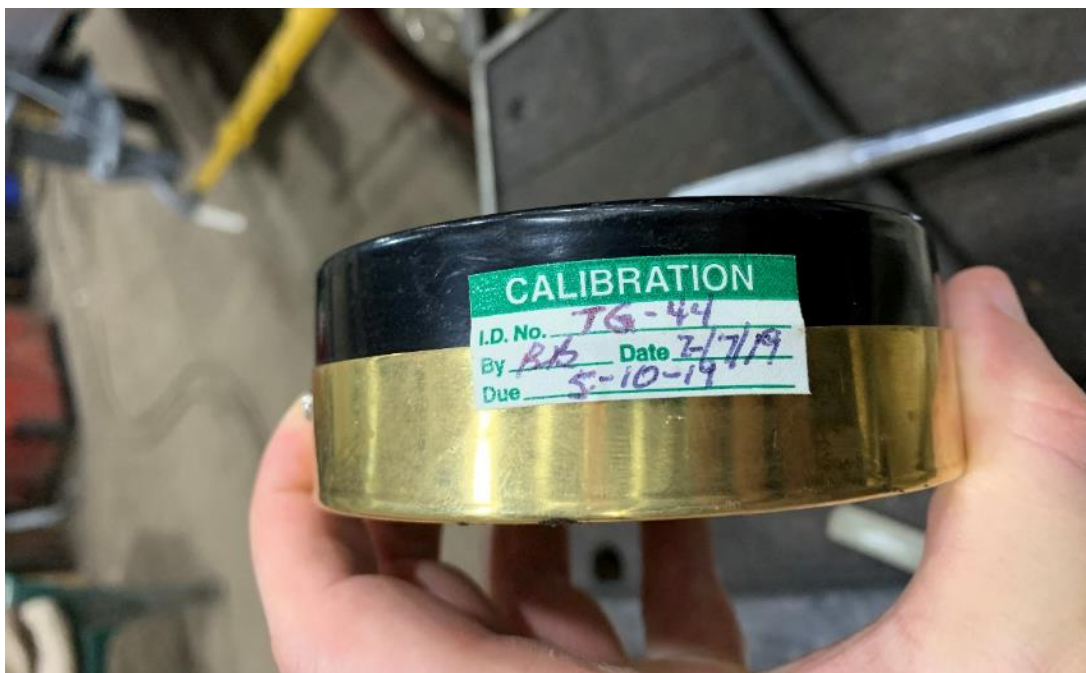
Figure C10. Brake Cylinder Pressure Gauge Calibration Information
