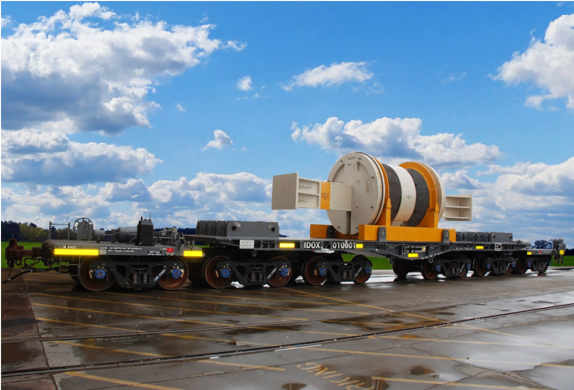
Figure 1. IDOX 010001 during Testing with Minimum Test Load
