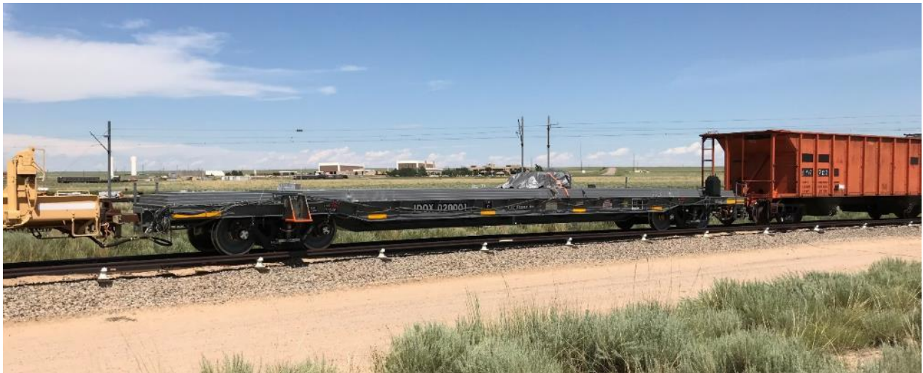
Figure 1. Buffer railcar IDOX 020001 during static testing
