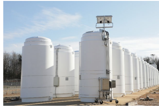
Fig. 1. HBURC in storage at the North Anna Power Station (front right). Source: DOE.
