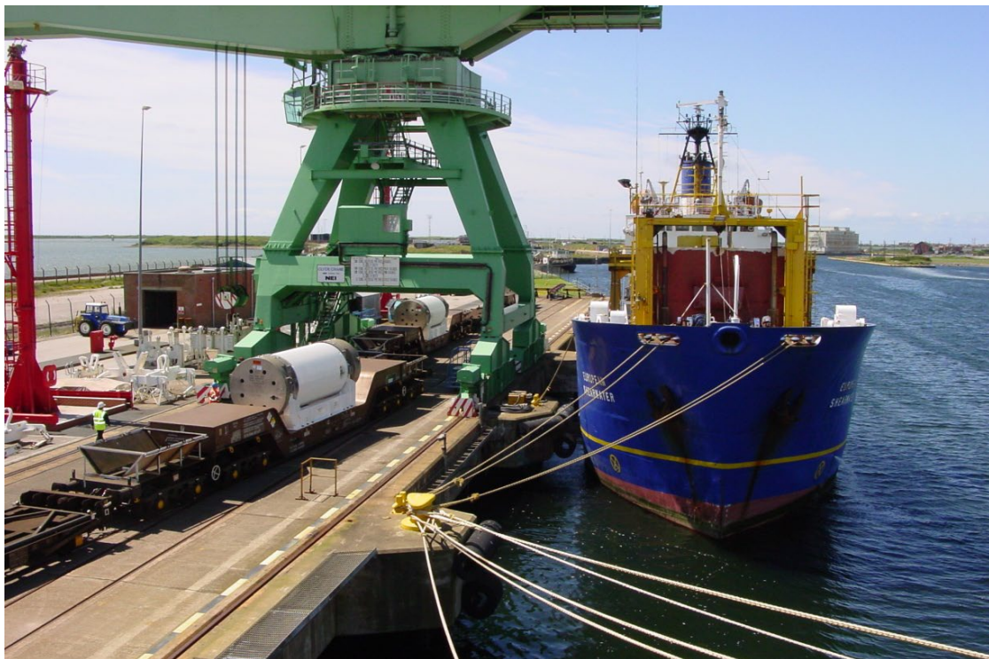
Fig. 2-1. Processing of casks between railcars and purpose-built vessel at Barrow-in-Furness. Photo by coauthor R. B. Pope during June 2002 IAEA appraisal of the safety of the transport of radioactive material for the UK (IAEA 2002).
