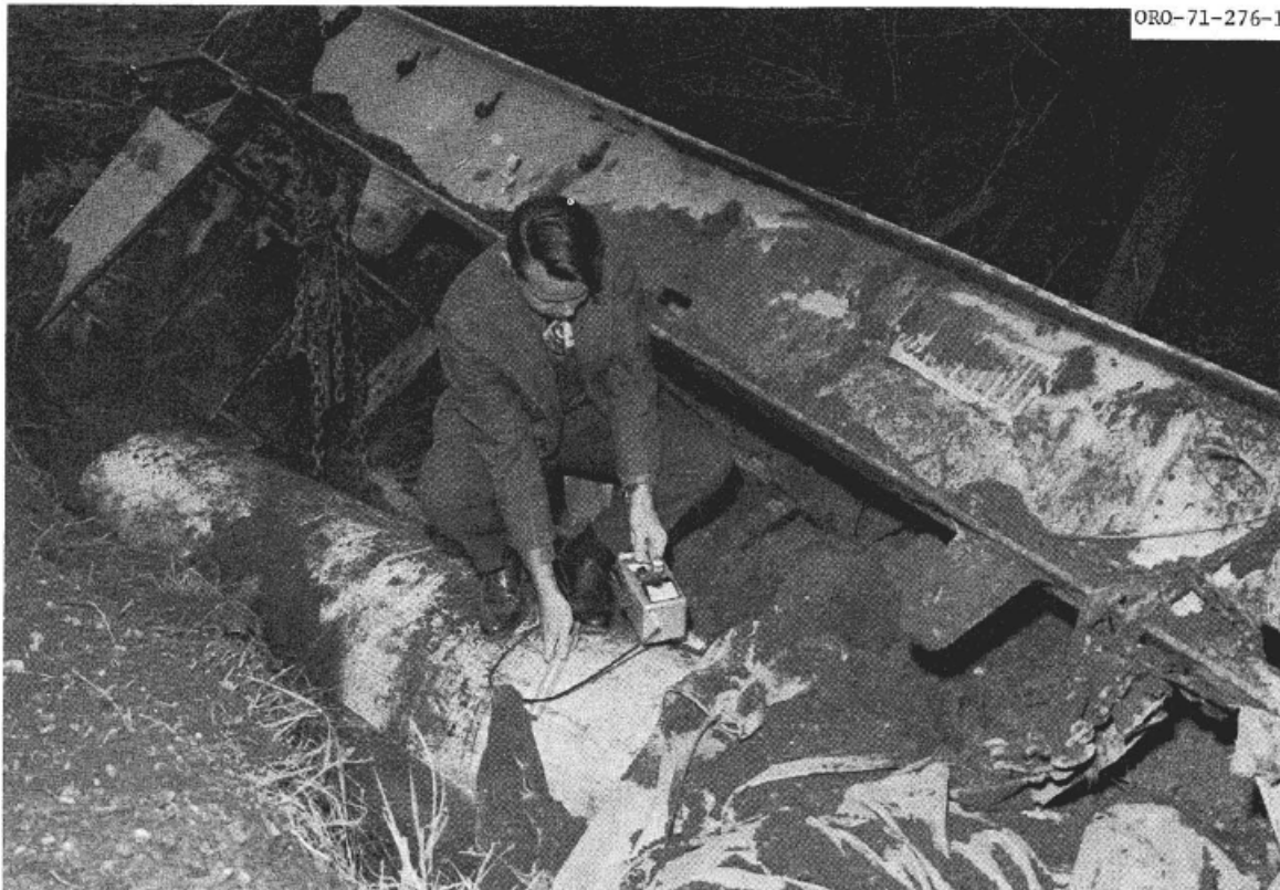
Fig. 4-3. Radiation survey performed on cask at accident site (Chandler 1972).
