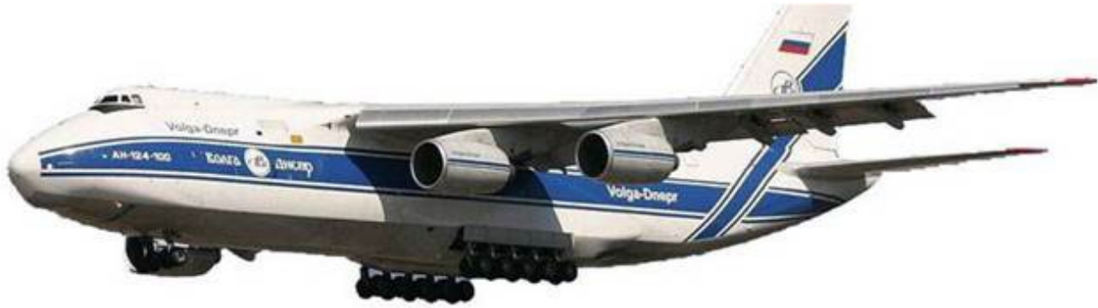
Fig. 2-21. AN-124-100 aircraft used for transport of TUK-19 casks (Bolshinsky 2010b).
