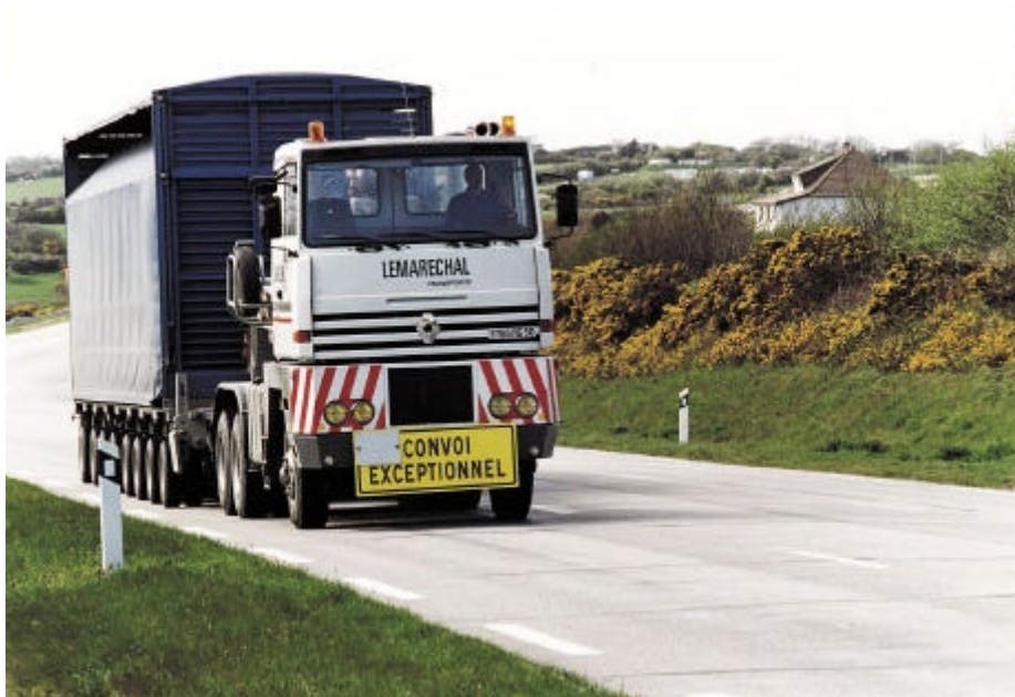
Fig. 2-13. Heavy-haul road transport of HLW cask between La Hague and Valognes, France (Verdier 2004).
