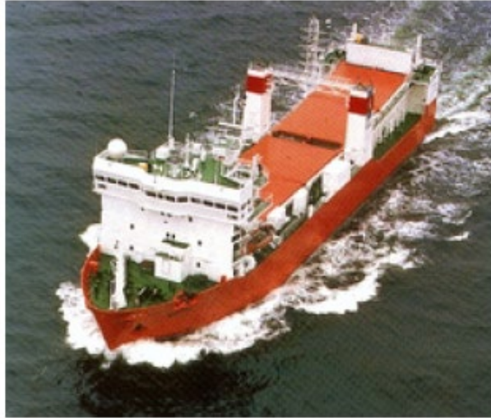
Fig. 2-2. M/S Sigyn, specially designed Swedish vessel for SNF and HLW transport (Posiva 2016).
