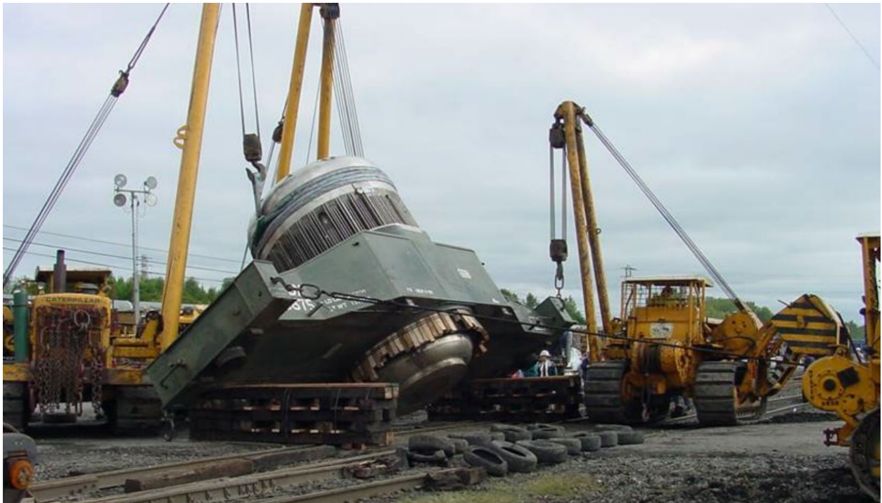
Fig. 3-1. Recovery of the SNF cask and railcar that derailed September 22, 2005.
