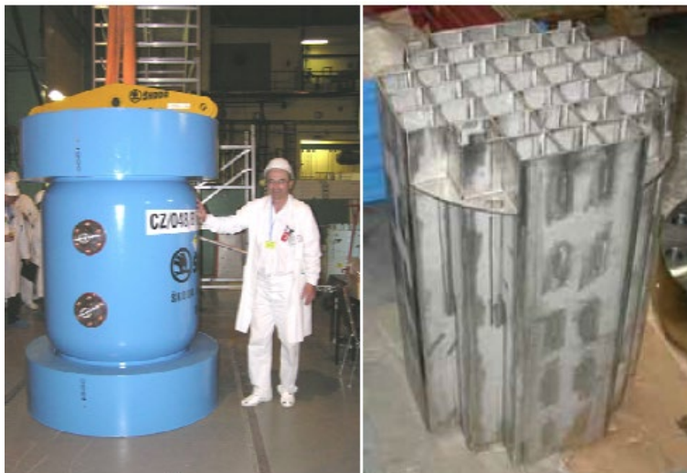
Fig. 2-22. SKODA VPVR/M cask and cask basket used for shipments from Czech Republic to Russia (Podlaha 2013).
