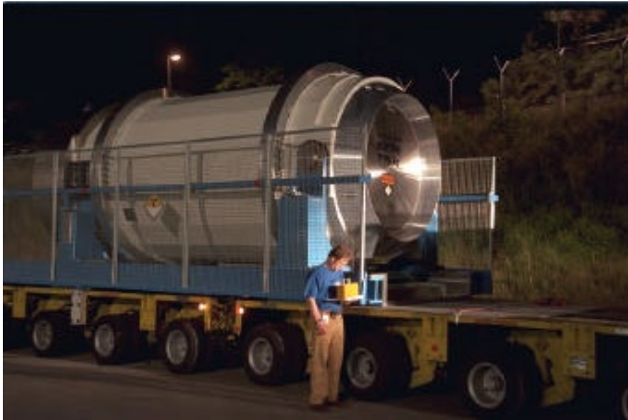
Fig. 2-10. The TN 97L dual-purpose cask loaded on a heavy-haul road transport vehicle in Switzerland (Sicard 2001).
