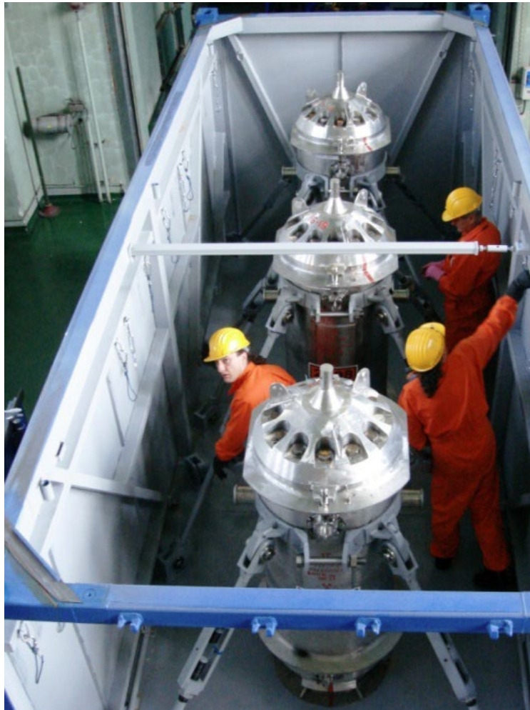
Fig. 2-20. Three TUK-19 casks loaded in a freight container prior to air transport (Bolshinsky 2010b).
