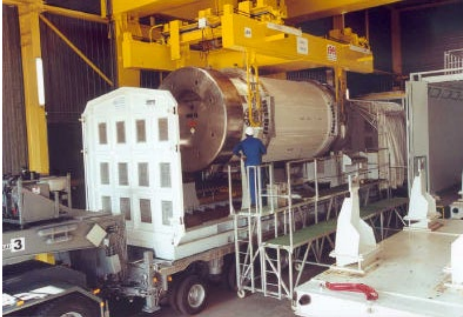
Fig. 2-8. TN 52L dual-purpose SNF cask being loaded onto a heavy-haul road vehicle (Roland 2001).
