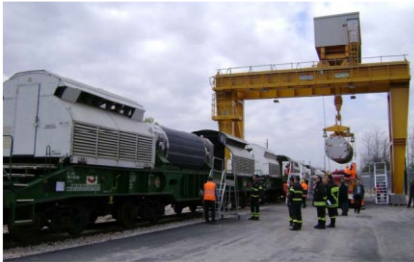
Fig. 2-18. Transfer of rail cask from heavy-haul road vehicle to railcar at the Caorso Multimodal Transfer point in Italy (Di Gasbarro 2010).
