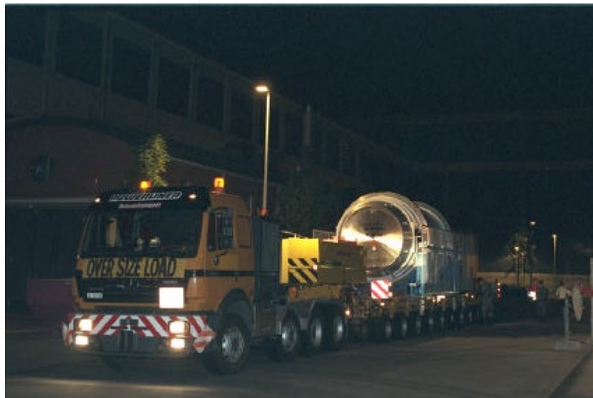
Fig. 2-9. TN52L dual-purpose SNF cask during transit on heavy-haul road vehicle (Roland 2001).
