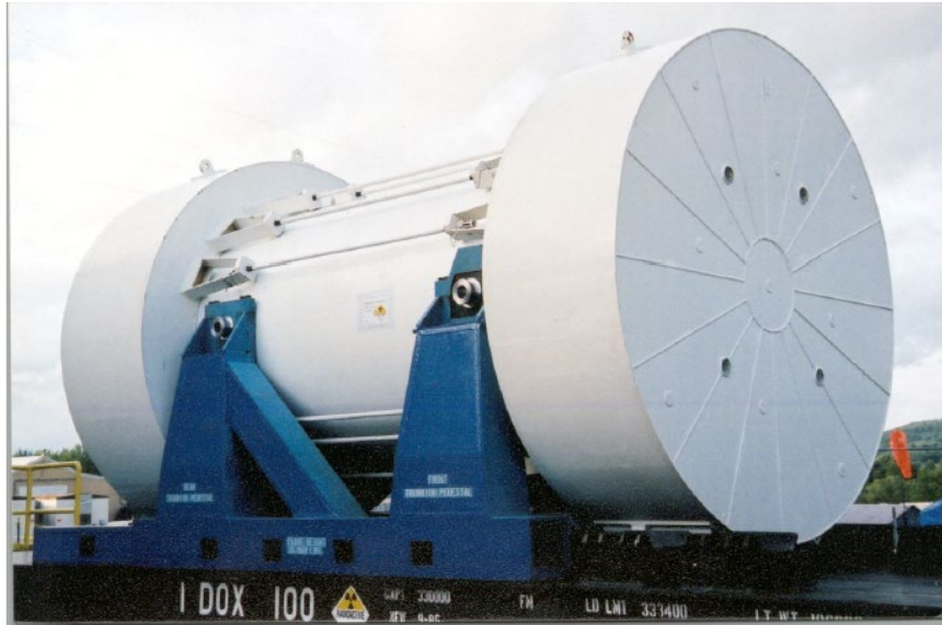
Fig. 2-16. Loaded West Valley cask with impact limiters and tie rods installed in 2003 (Tyacke 2004).
