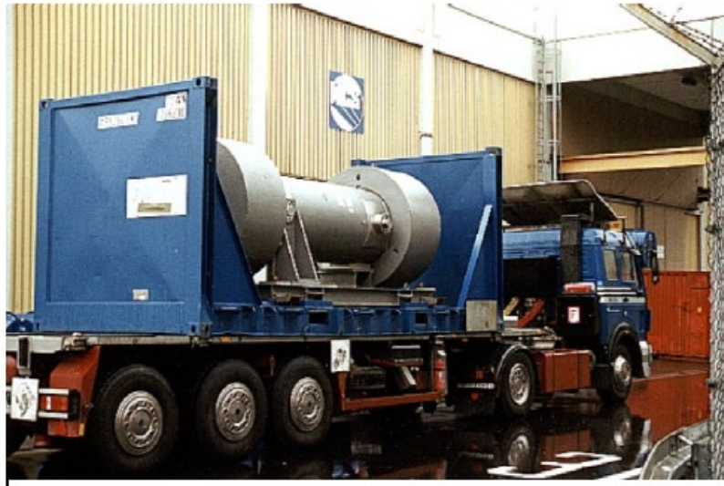
Fig. 2-6. TN 7-2 transport cask loaded on a road vehicle used for transport of research reactor SNF (Schmidt 2001).
