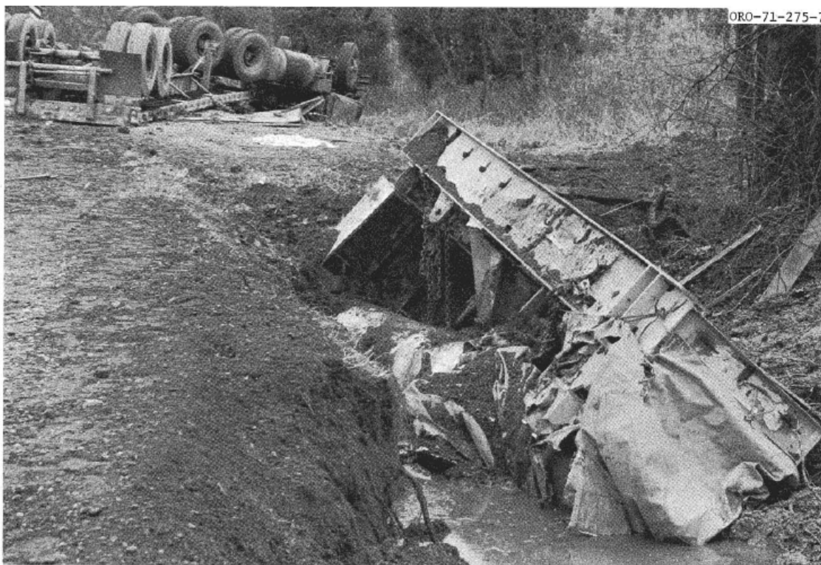
Fig. 4-2. Cask and skid separated from tractor-trailer (Chandler 1972).
