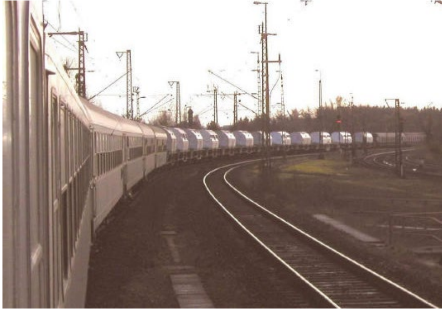
Fig. 2-14. Train consist containing 12 cask railcars and associated security personnel cars from La Hague to Germany (Verdier 2004).
