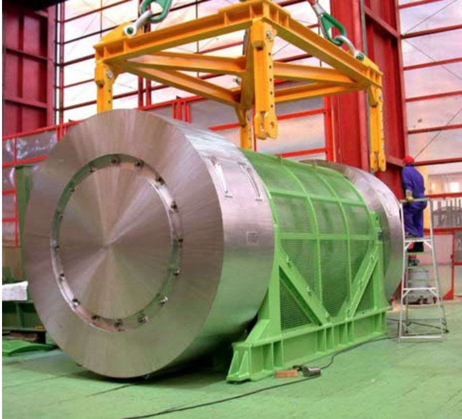
Fig. 2-11. NAC-STC on transport skid in China (Meinert 2001).
