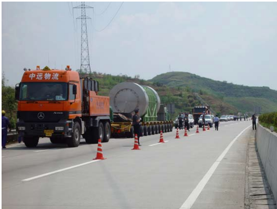
Fig. 2-12. NAC-STC cask in transit by highway in China (Meinert 2001).
