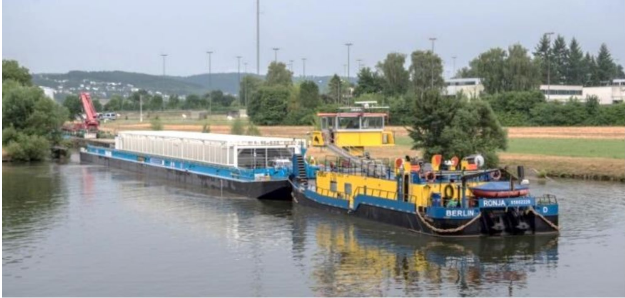
Fig. 2-23. Inland barge and pusher tug transporting SNF by inland waterway in Germany (Pätzold and Köbel 2019)
