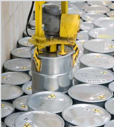
A loading crane is used for waste handling.
