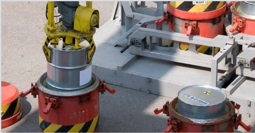
Radioactive waste with a high radiation dose on the surface of the drums is transported in shielding containers.
