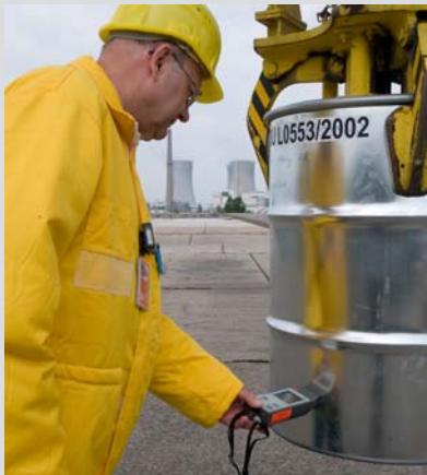
Measurement of the radiation dose on the surface of a drum.
