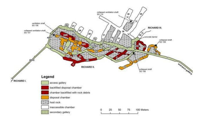
**The repository Bratrství** is located in a former uranium mine near the town of Jáchymov and is designed for disposal of waste containing naturally occurring long-lived nuclides only, such as <sup>226</sup>Ra and uranium. Its disposal capacity is approx.1 200 m<sup>3</sup>, from which is free approx. 340 m<sup>3</sup>. In 2012 the chamber 2 was sealed with special concrete backfill. Sealing of the remaining chambers will follow.
