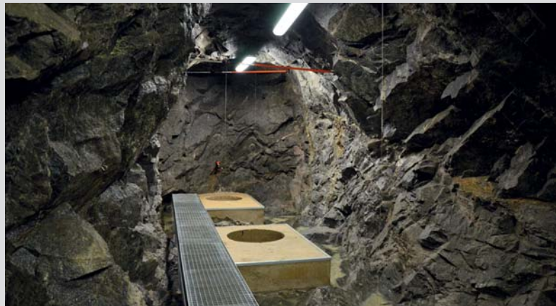
Preparation of an in-situ experiment simulating the vertical emplacement of a spent nuclear fuel container.
