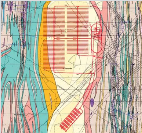
Geological conditions at a depth of 500 metres - Kraví hora - Spatial layout of a repository.
