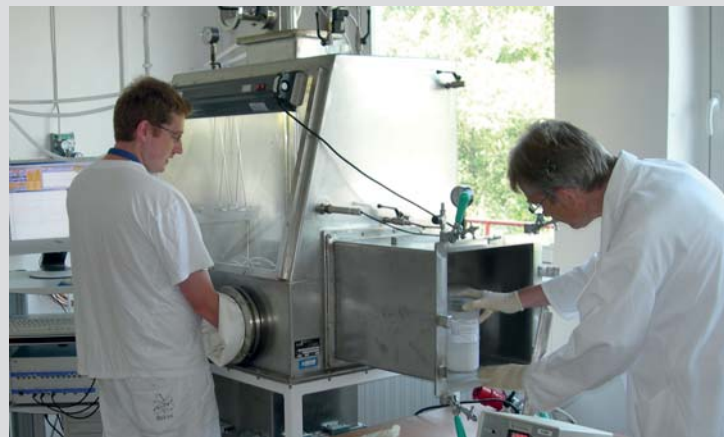
Glove box with an integrated high-temperature electrolyzer.
