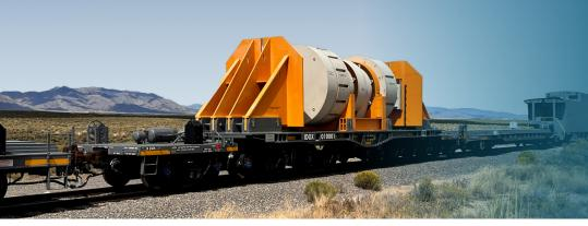
The U.S. Department of Energy (DOE) is developing special railcars for future large-scale DOE transport of spent nuclear fuel (SNF) from nuclear power plants. The designs include new buffer railcars, the Atlas railcar (designed to transport SNF containers), and a new escort railcar for security personnel that was developed in collaboration with the U.S. Navy.
