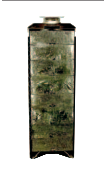
Cut-away model of a CSD-C container showing the stack of wafers
