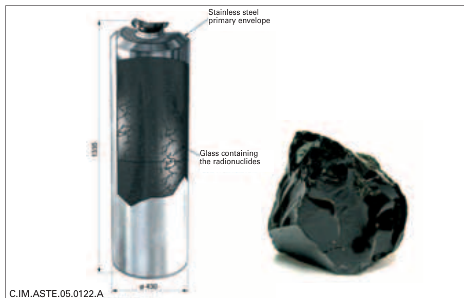
Diagram of an R7T7 vitrified C waste primary package
