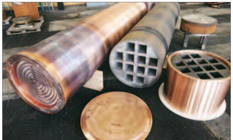
Copper container demonstrator tested by the Swedish organisation SKB
