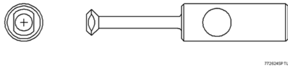
Figure 11-10 Bushing Extractor (P/N 772624)
