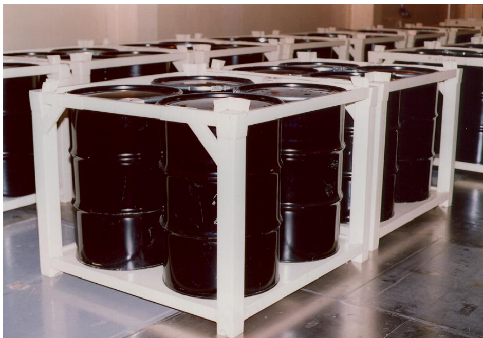
Storage of low and intermediate level waste
