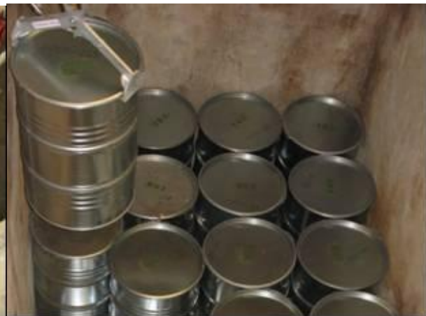
Storage of re-packed wastes
