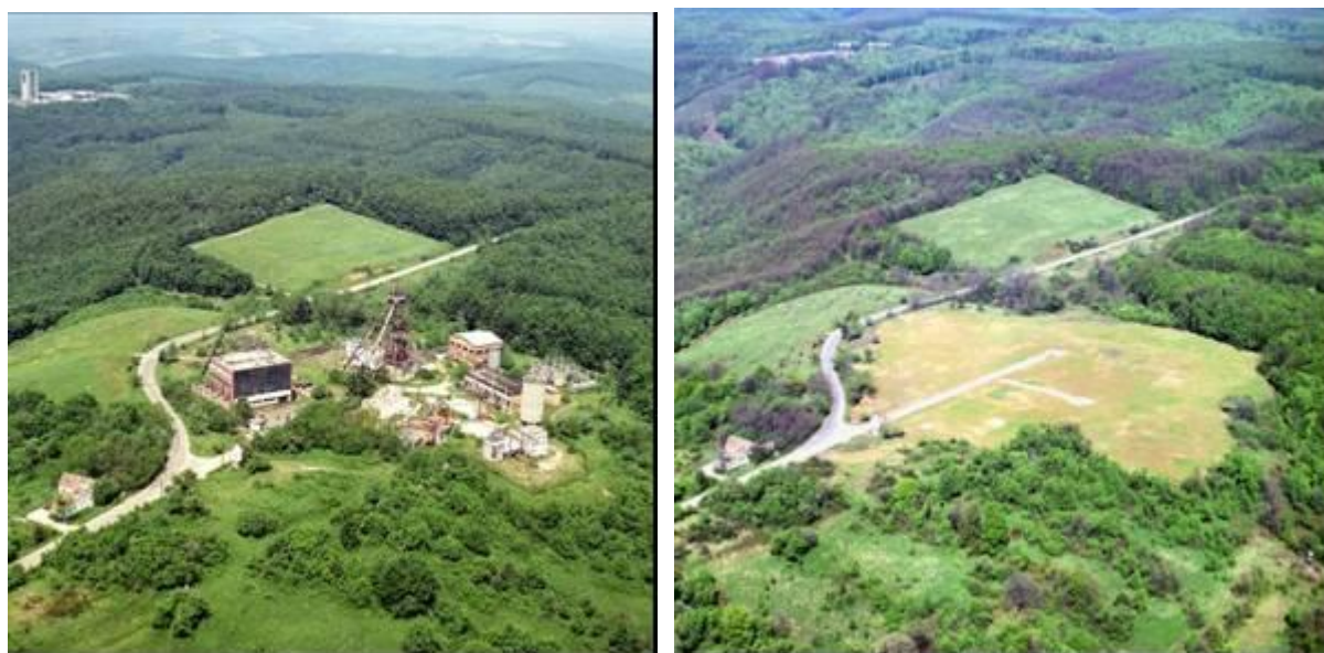
Air shaft IV of the uranium ore mine during operation and after remediation
