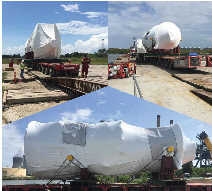
Figure 3-13: Large Components Arriving at CR-3 by Barge [31]
