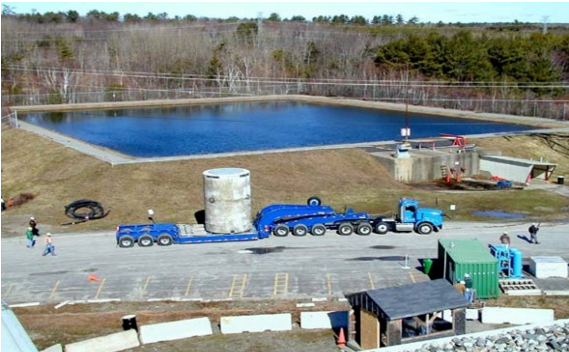
Figure 2-37: Loaded VCC on HHT
