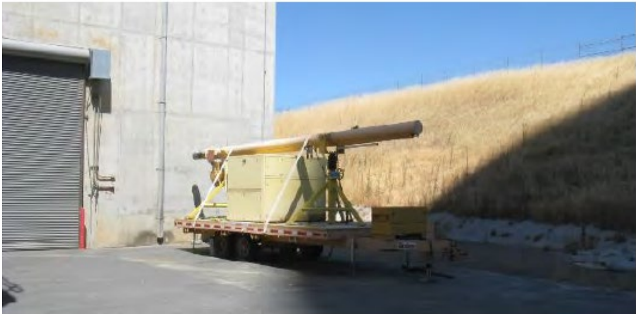
Figure 2-7: Hydraulic Ram System Used to Emplace and Withdraw Canisters from HSMs at Rancho Seco (2013) [10]
