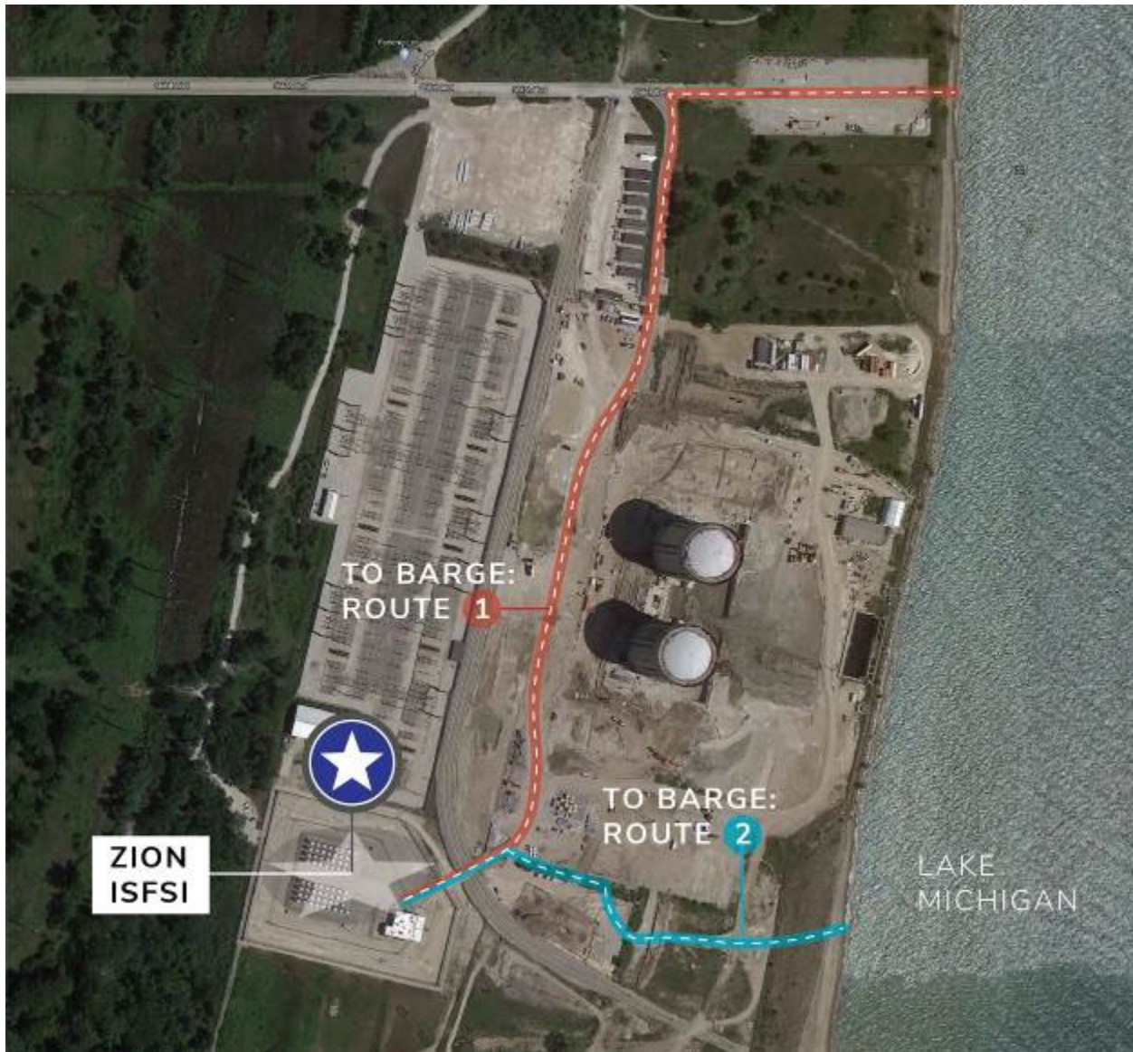
Figure 3-3: Zion Potential Barge Loading Sites
