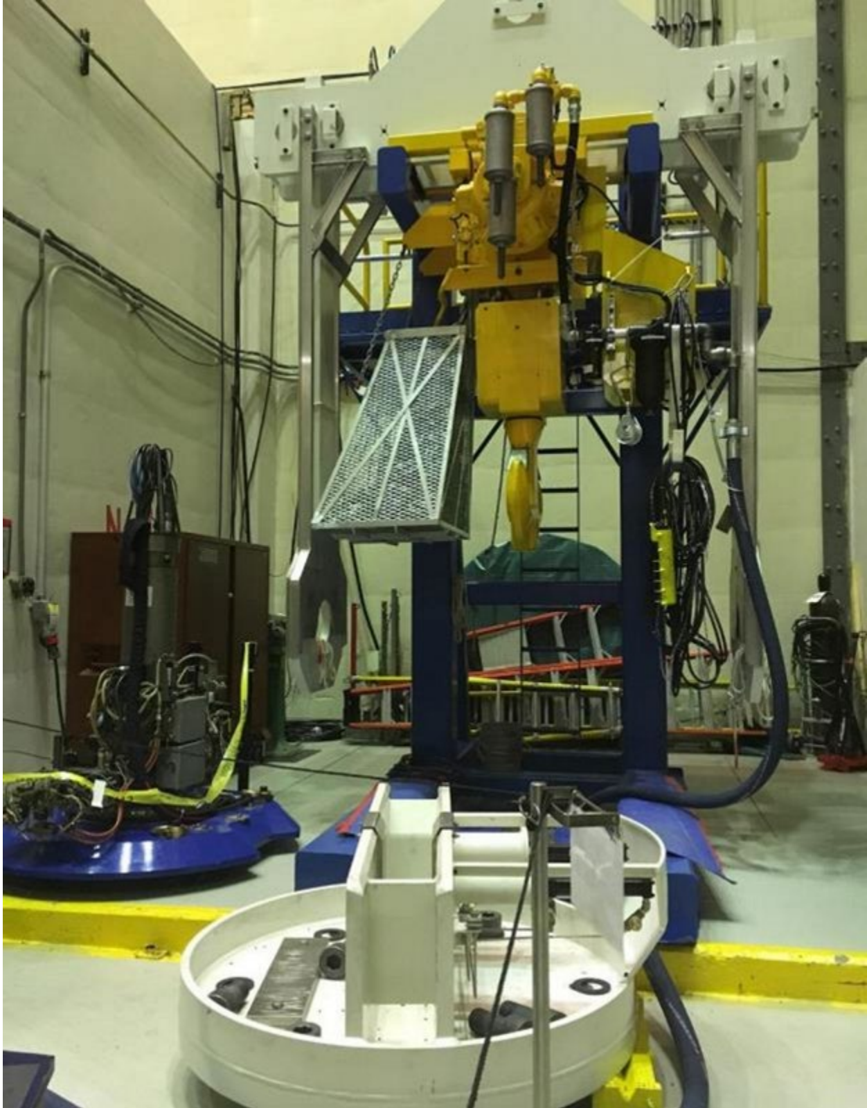
Figure 2-35: MAGNASTOR Secure-Lift Yoke and Chain Hoist with TSC Lift Adapter Plate
