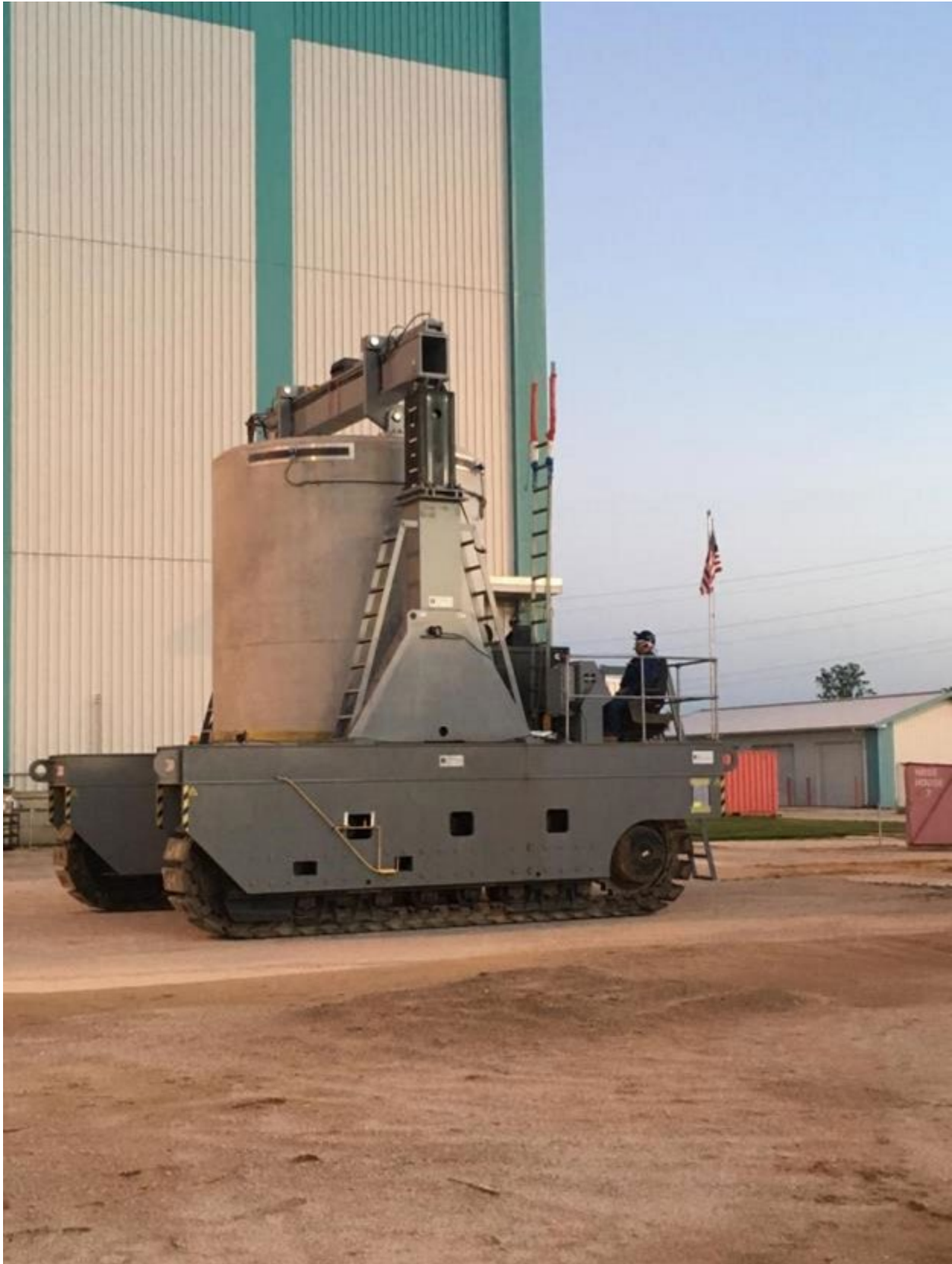
Figure 2-32: MAGNASTOR VCC Engaged to Self-Propelled VCT
