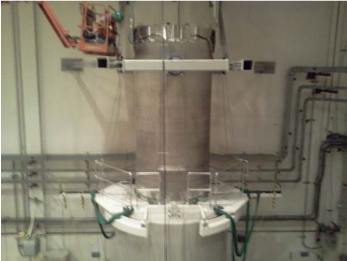
Figure 2-22: MAGNASTOR Transfer Cask (MTC) [19] Transfer of Zion TSC into VCC with MTC Restraints Installed
