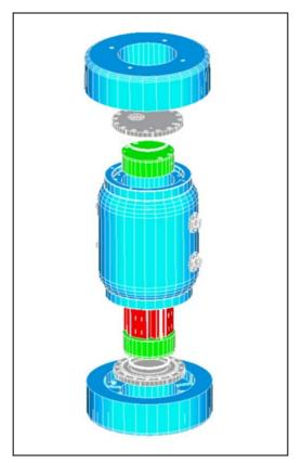
Fig. 11.1 Škoda VPVR/M cask with shock absorbers, basket, primary and secondary lids
