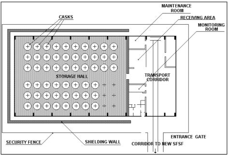
Fig. 4.2 Ground plan of ISFSF Dukovany
