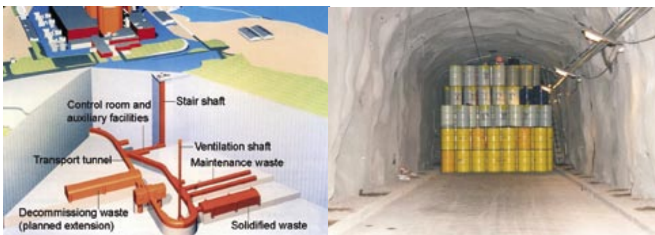
Figure 5. The left picture gives a cross-sectional view of the repository for LILW and the planned extension for decommissioning waste and in Loviisa. The right photograph illustrates the drums of low level maintenance waste in the repository tunnel.
