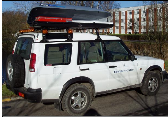
Figure 9. Mobile measurement system equipped with a 4L NaI(Tl) and a GR-320 spectrometer.
