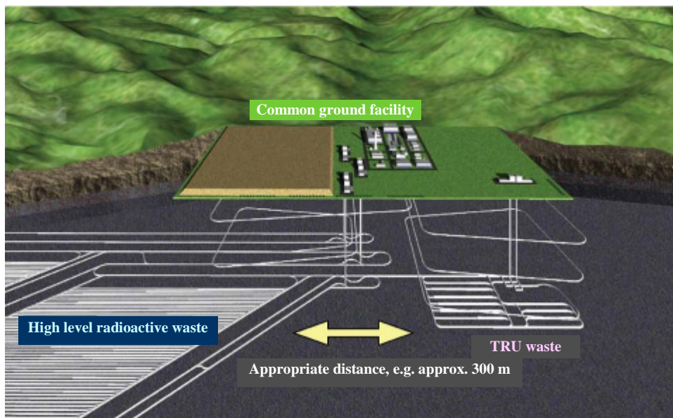
Fig. L6-4-2 Concept of single-site disposal (Source: Home page of the Agency for Natural Resources and Energy)
