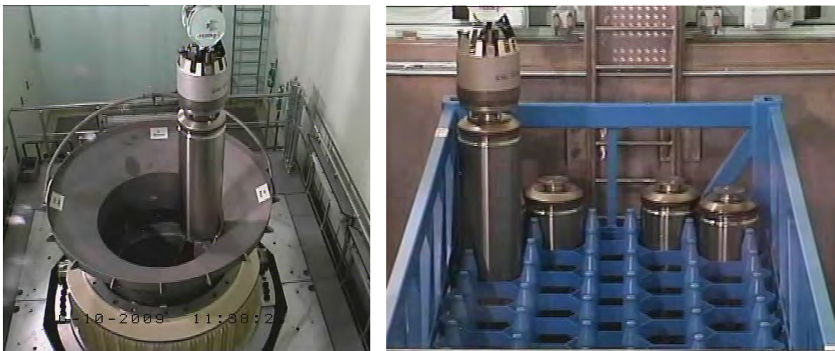
Figure 4 and 5: Transshipment of CSD-C canisters with compacted structural elements from a transport cask to a storage container at the Central Storage Facility (ZZL) in Würenlingen (Photos: Zwiilag).
