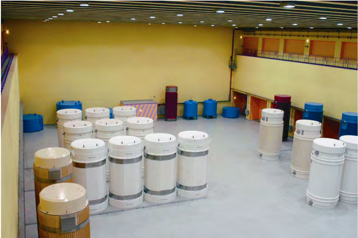
Figure 8: Transport and storage casks in the hall for dry storage Central Storage Facility ZZL (Photo: Zwiilag)
