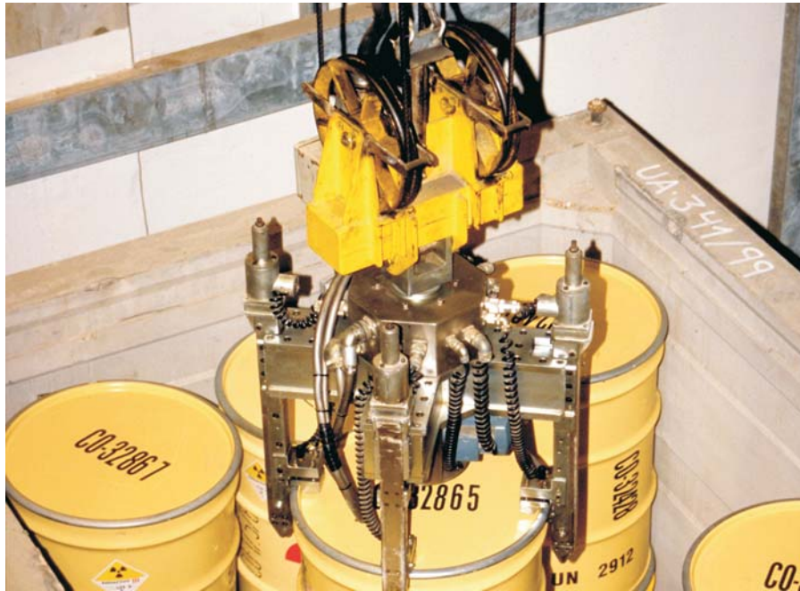
Radioactive waste management facilities: disposal of drums conditioned in containers (El Cabil).
