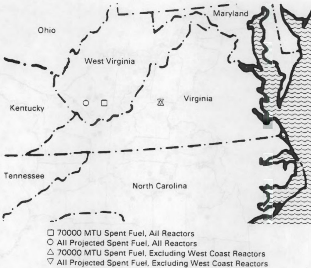
FIGURE D.3. Geographic Centroids of Projected Spent Fuel Shipments to an MRS Facility
