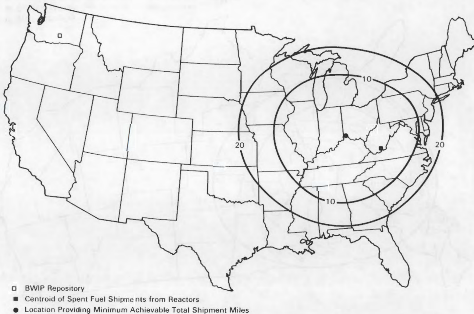
FIGURE 6.3. Minimum Distance Contours Assuming Single-Cask Shipments to and from the MRS Facility, Spent Fuel Rod Consolidation (2:1), and the First Repository at BWIP
