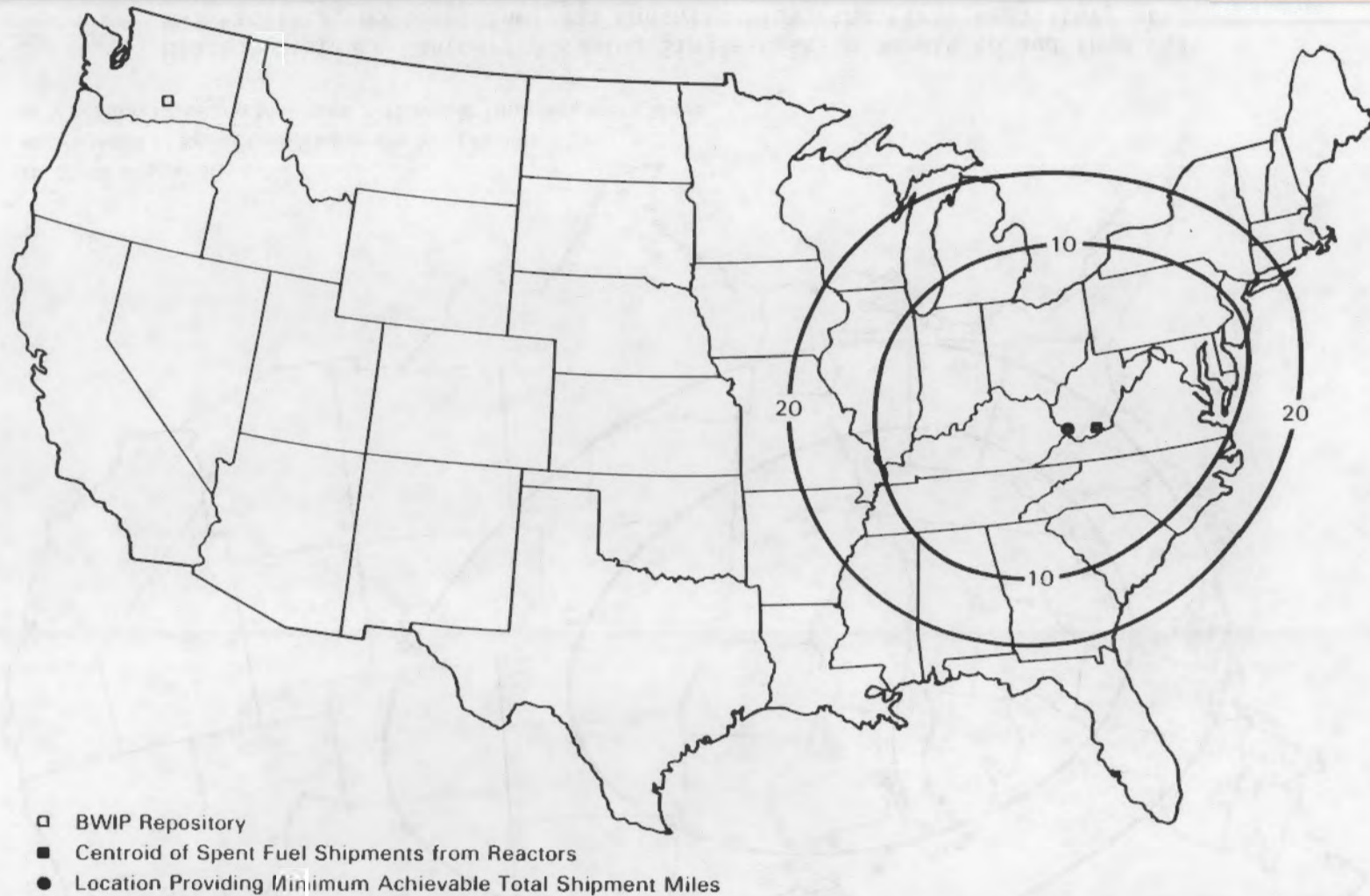
FIGURE 6.5. Minimum Distance Contours Assuming Single-Cask Truck or 3-Cask Rail Shipments to the MRS Facility, 5-Cask Shipments from the MRS Facility, No Spent Fuel Rod Consolidation, and the First Repository at BWIP
