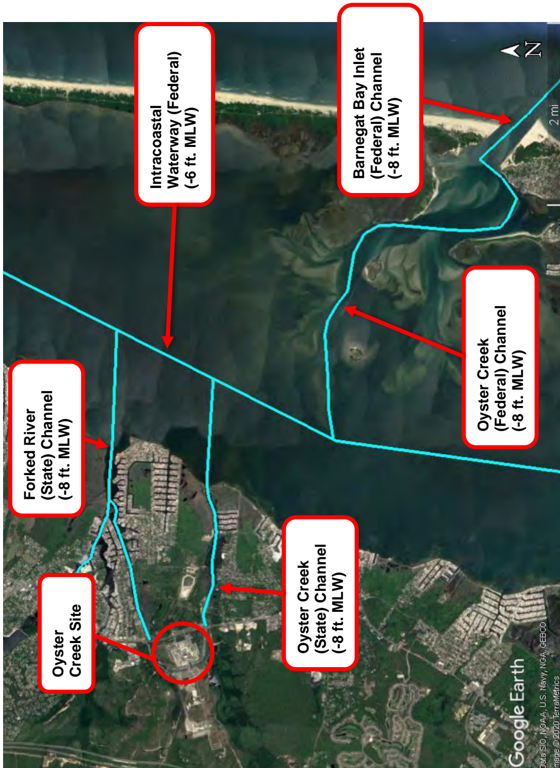
Figure 2-403. Aerial View of the Oyster Creek State and Federal Channels, the Intracoastal Waterway, and the Barnegat Bay Inlet Channel (Google 2022)
