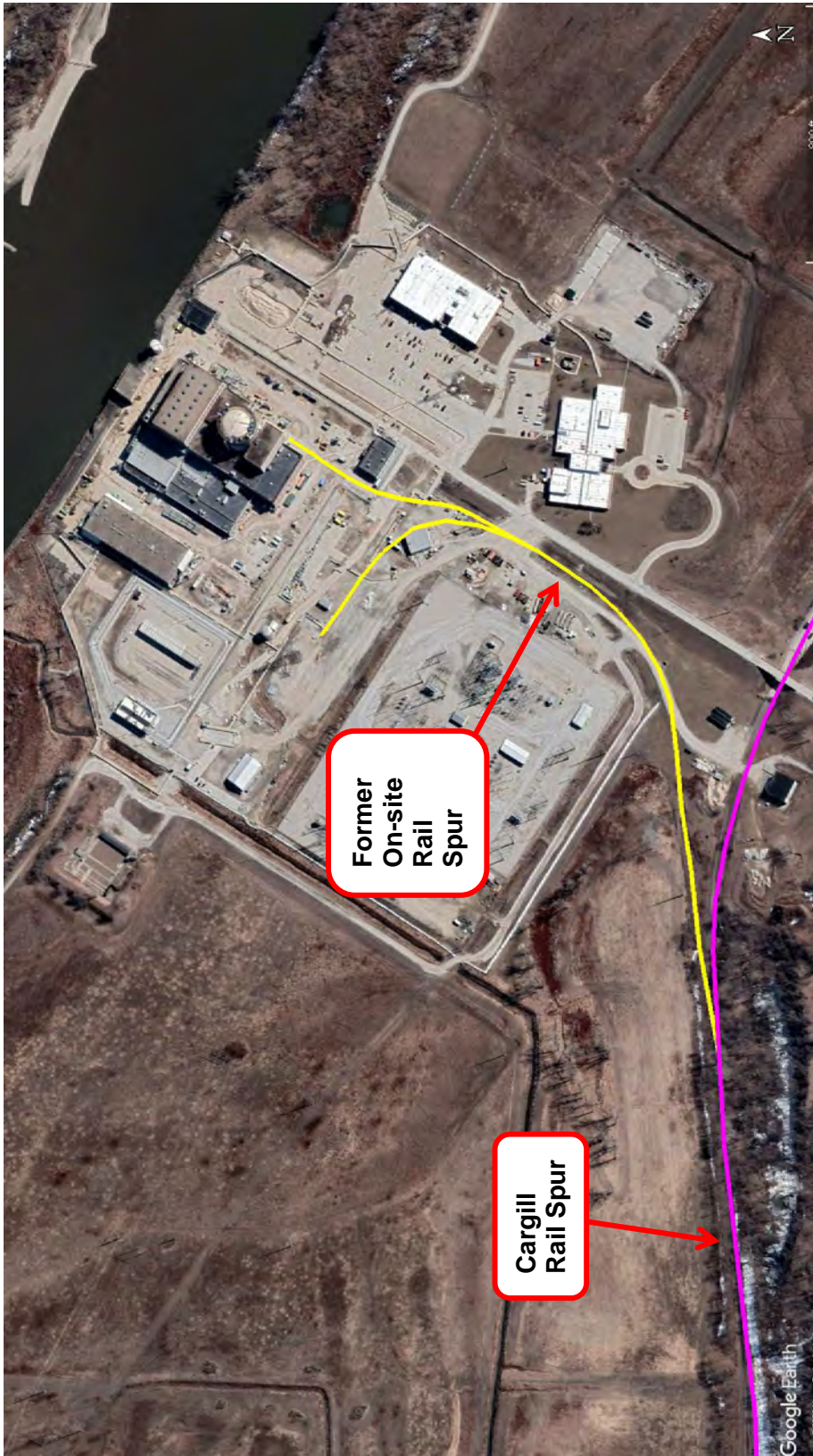
Figure 2-351. Former On-site Rail Spur at Fort Calhoun (Google 2022)
