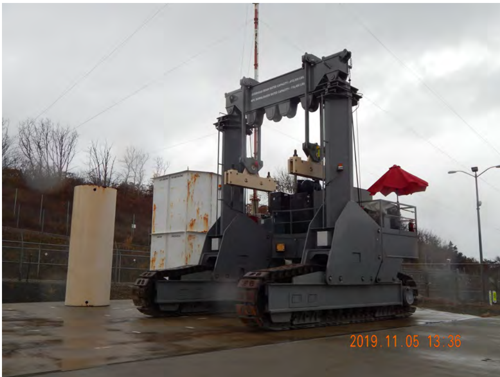
Figure 2-409. Storage System Mover at Pilgrim Independent Spent Fuel Storage Installation (2019)
