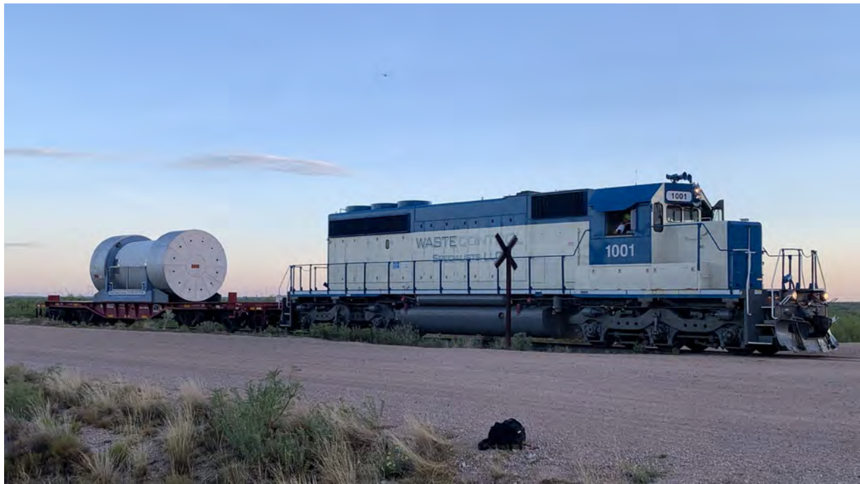
Figure 2-341. MP197HB Transportation Cask Carrying Segmented Reactor Internals from Vermont Yankee Arriving at the Waste Control Specialists Low-Level Radioactive Waste Disposal Facility in Andrews, Texas (2020)
