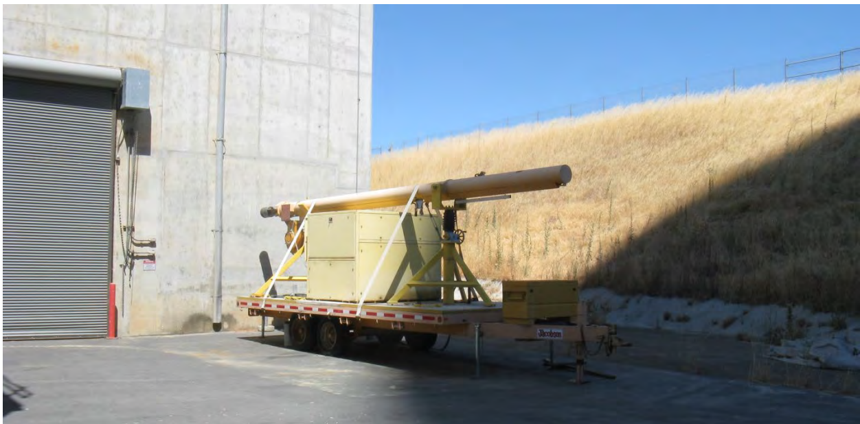
Figure 2-86. Hydraulic Ram Used to Emplace and Withdraw Canisters from Horizontal Storage Modules at Rancho Seco (2013)
