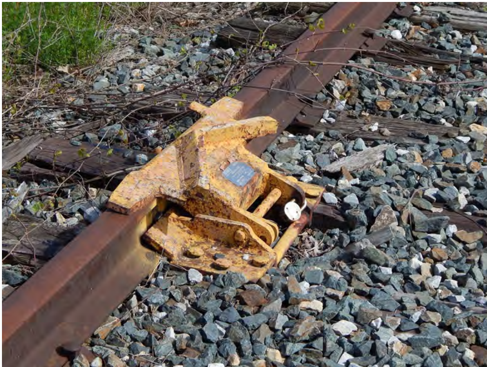
Figure 2-330. Derailer on Vermont Yankee Rail Spur (2016)
