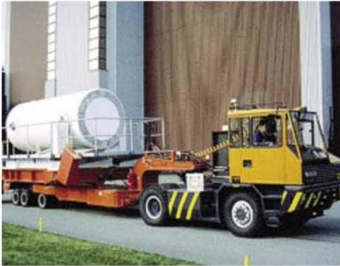
When the spent fuel is taken out of the reactor it cools down in the reactor hall for few years. After that the spent fuel is transported to the interim storage located on the plant site.
