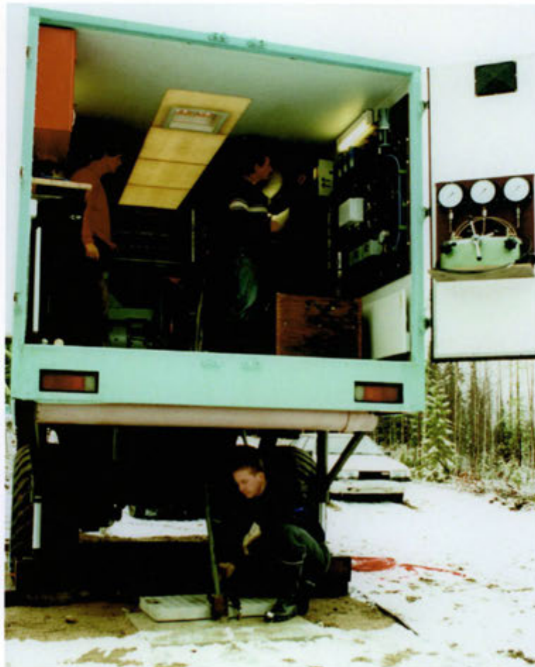
Figure 2.3-3. Hydraulic testing unit (HTU) mounted on a trailer. The data acquisition and processing equipment are in a separate compartment in the front part of the trailer. The hydraulic cable winch and instruments for measurement, control and operating can be seen in this picture. The cable is lowered into the borehole through a hatch in the floor.
