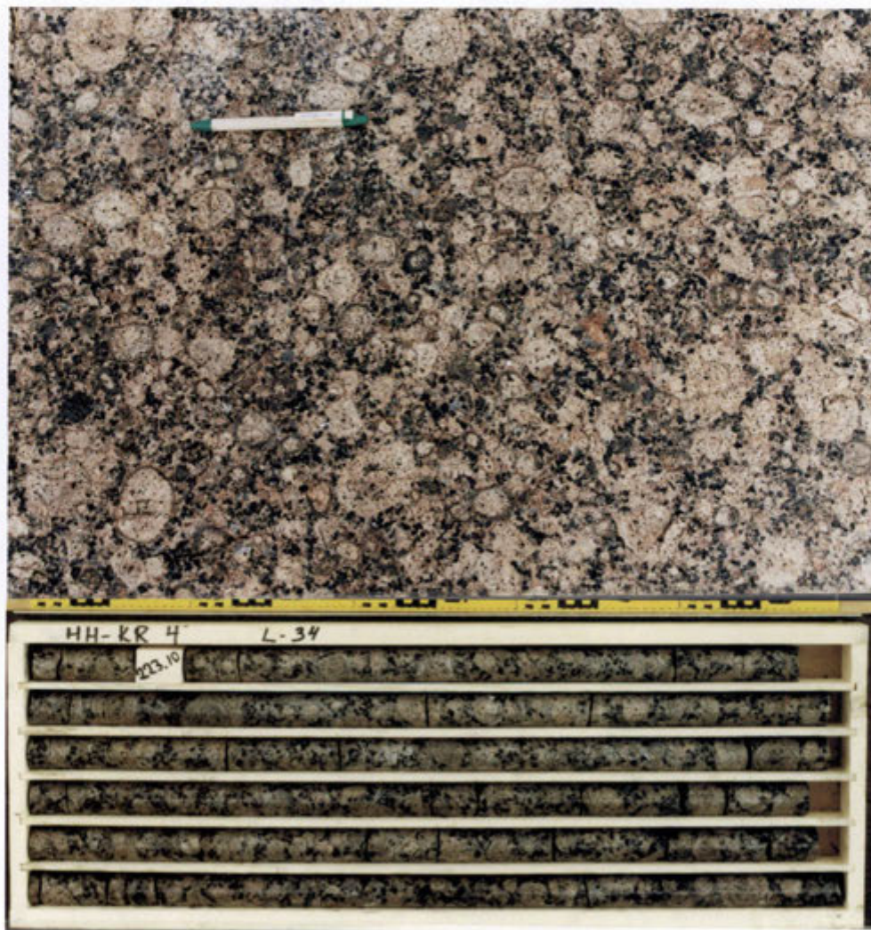
Figure 4.1-2. Pyterlite on the outcrops and as core drilled rock samples.
