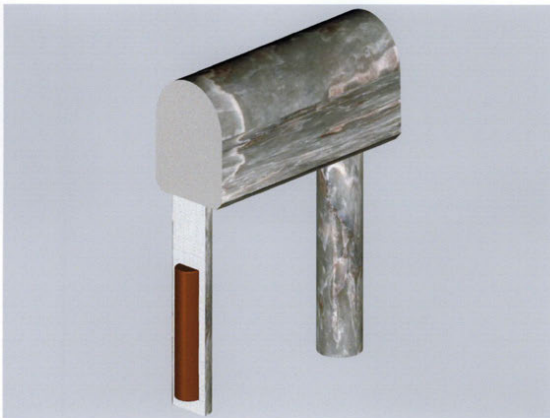
Figure 9.1-2. Backfilled deposition tunnel with a canister in the disposal hole.
