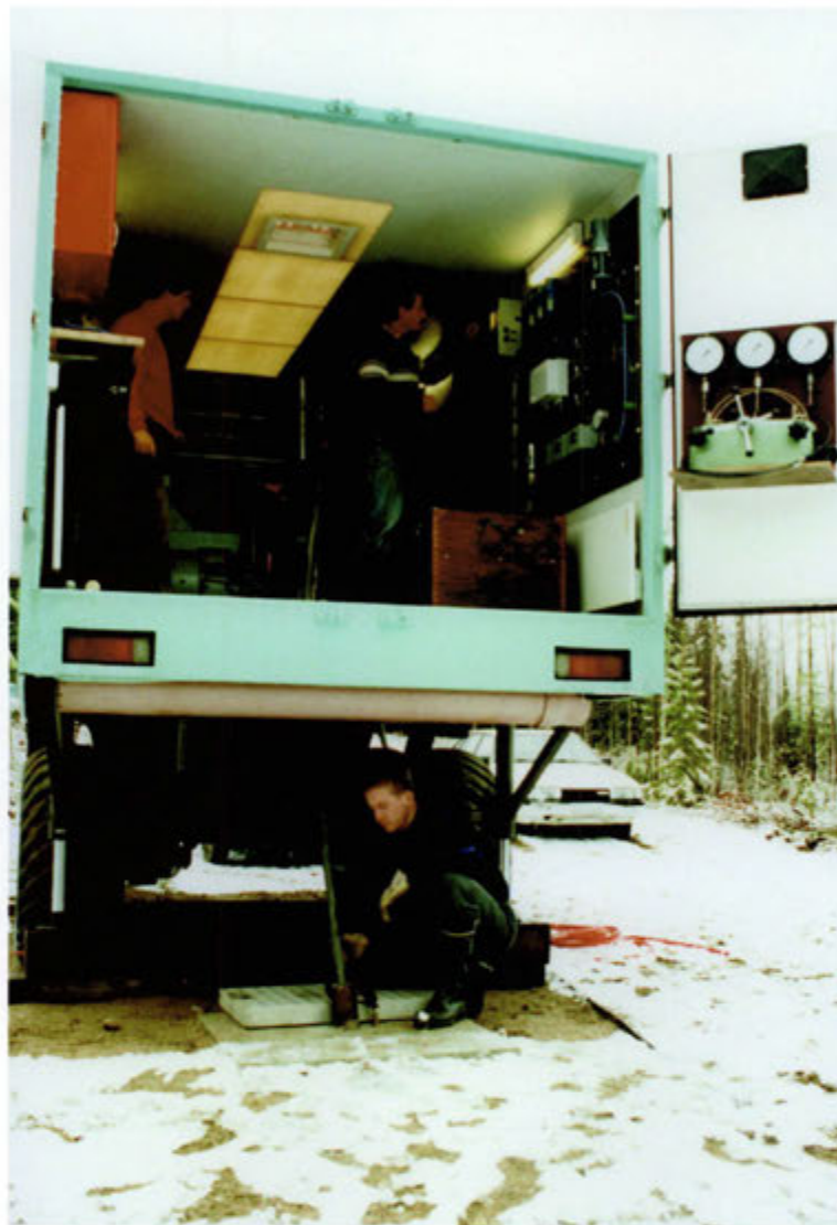
Figure 2.2-7. Hydraulic testing unit (HTU) mounted on a trailer. The data acquisition and processing equipment are in a separate compartment in the front part of the trailer. The hydraulic cable winch and instruments for measurement, control and operating can be seen in this picture. The cable is lowered into the borehole through a hatch in the floor.
