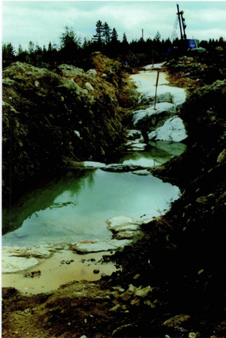
Figure 2.3-2. Investigation trench TK1 seen from SW. The drilling rig behind the trench is on the borehole KR2. In the depression in front the fracture zone R11 crosses the trench. The trenches were landscaped after completion of the mapping.
