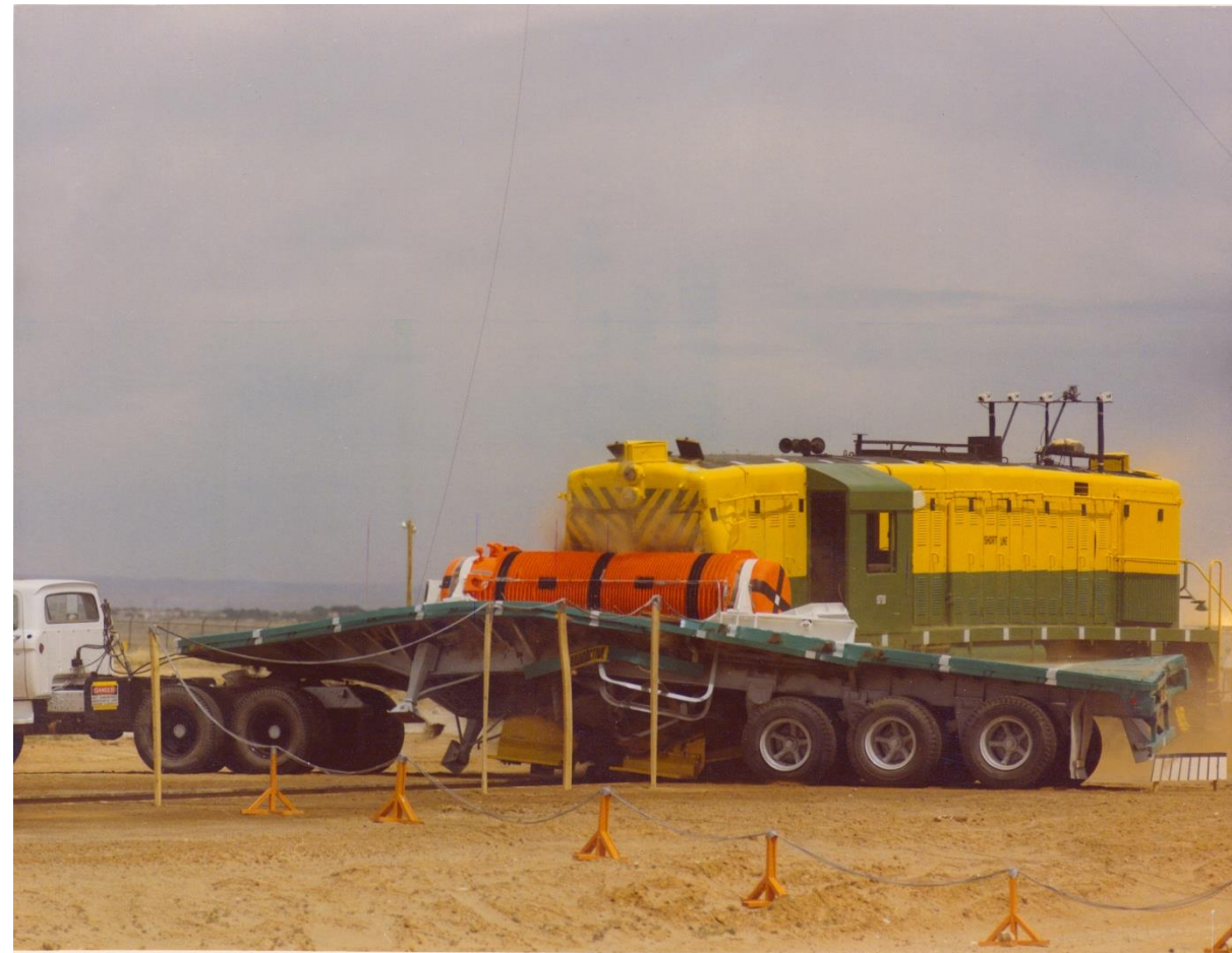
A photo showing a Sandia National Laboratories package performance demonstration with a train colliding with a cask on a flatbed trailer. Image courtesy of Sandia National Laboratories.
