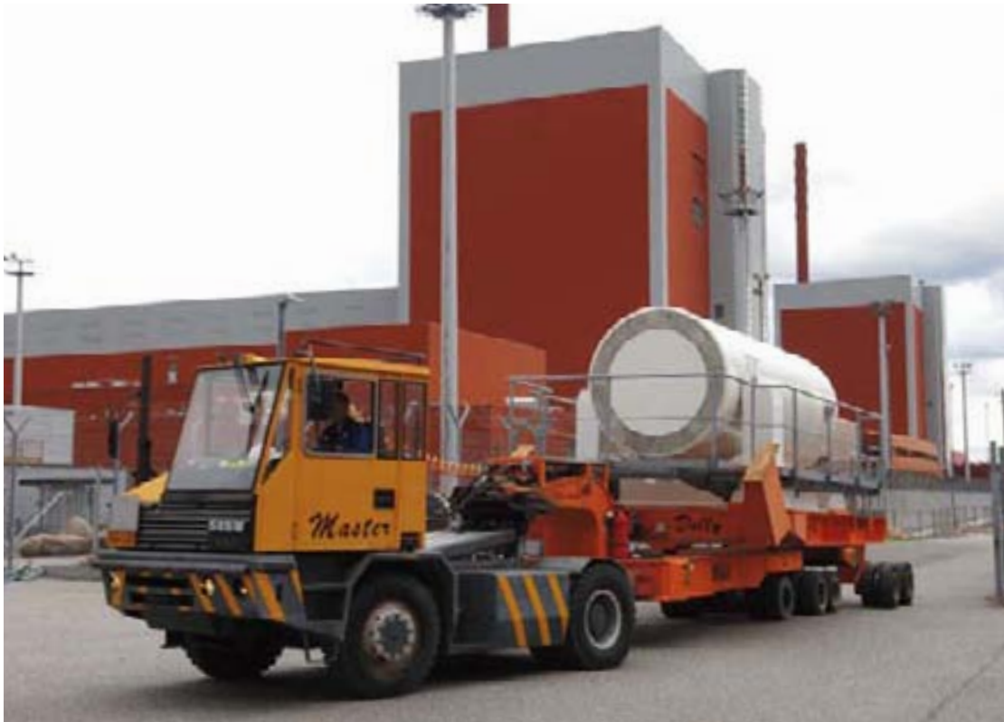
Figure 3-6 A transportation vehicle and container for spent nuclear fuel, with which fuel is transferred in the Olkiluoto power plant area.
