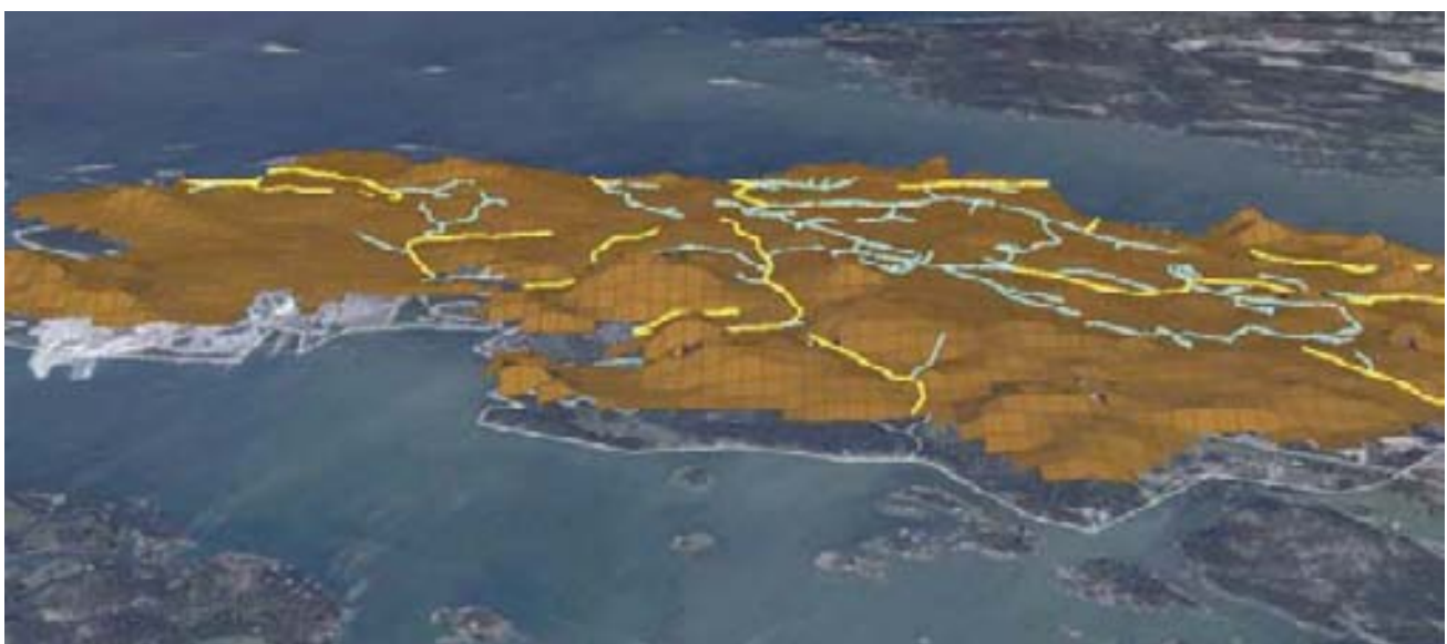
Figure 8-7 Uplift (exaggerated) and ditch network of Olkiluoto Island.
