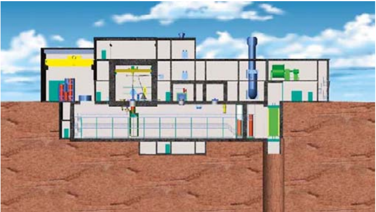
Figure 3-8 The encapsulation plant. Spent nuclear fuel transported to the plant will be packed into disposal canisters. The canisters will be sealed and transported to the repository using the lift shaft or access tunnel.
