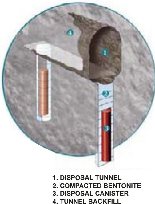
Figure 3-2 Multi-barrier principle for final disposal. Different barriers back-up each other.
