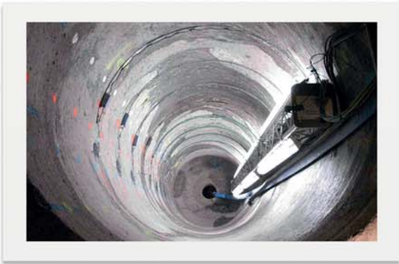
Experiment in a test hole to study the spalling strength of Olkiluoto rock in ONKALO.
