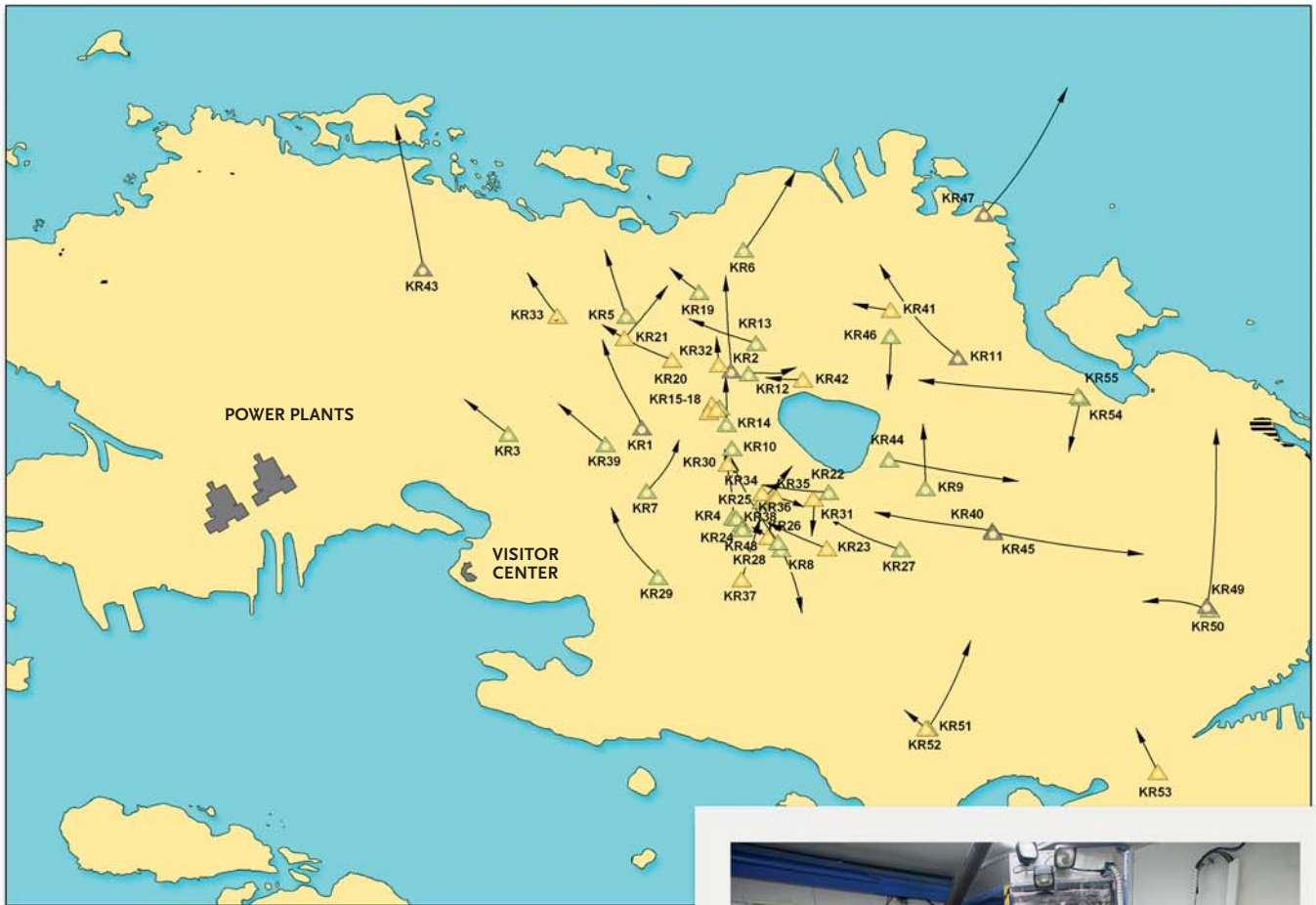
Investigation site for final disposal in Olkiluoto. More than 50 deep drillholes have been drilled in the area since the late 1980's.
