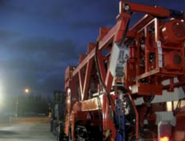
The boring machine "Sanna" will be used in the boring of full-scale canister deposition holes to test the final disposal technology.
