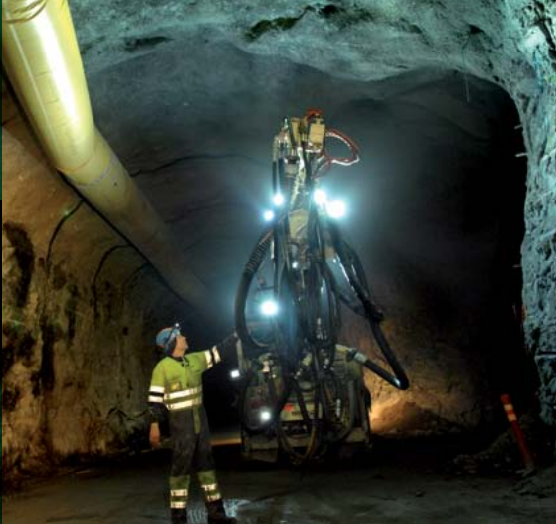
A machine used to inject a concrete mix at the technical level of ONKALO. ▶
