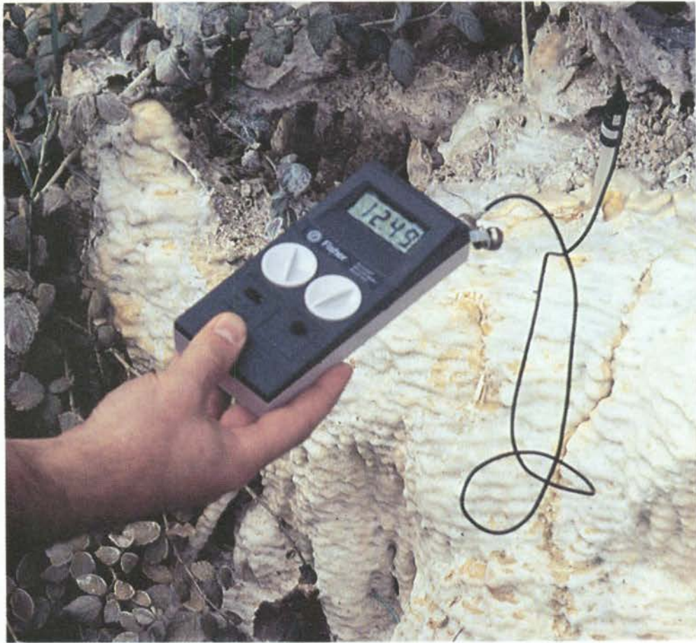
Figure 8-12. Measurement of pH in the hyperalkaline groundwater at Maqarin.
