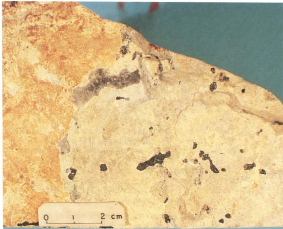
Figure 8-6. Phonolite from the Osamu Utsumi uranium mine in Poços de Caldas. The sharp boundary between oxidized rock (grayish-brown) and reducing (gray) can be seen. The black nodules on the reducing side are the uranium ore pitchblende.
