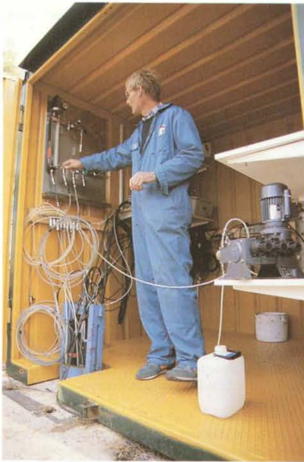
Figure 11-2. Different types of tracer tests are performed in or between boreholes down to a depth of 1 000 m. The picture shows injection of tracer in such a test.
