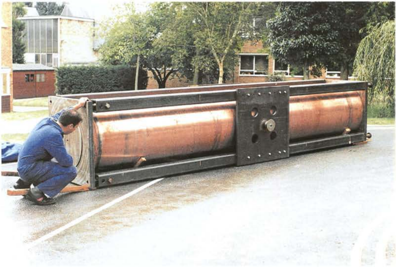
Figure 6-3. Full-scale canister produced during fabrication trials with self-supporting inner steel canister.
