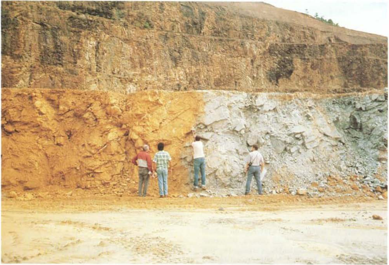
Figure 11-1. Sampling at a redox front in the Osamu Utsumi uranium mine for analysis of the minerals.
