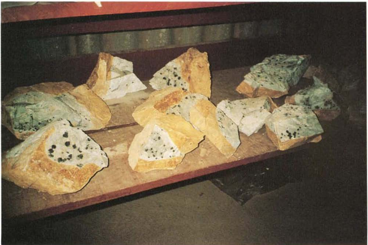
Figure 11-2. Rock samples from the redox front. Precipitations of uranium in the form of pitchblende can be clearly distinguished as black spots.
