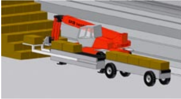
Figure 15-3. Rig for transport and installation of blocks.
