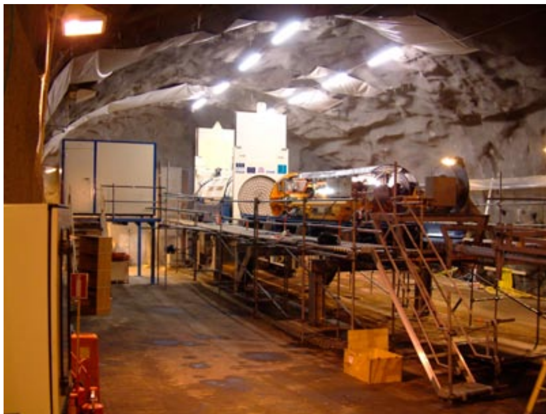
Figure 18-3. KBS-3H – deposition equipment in the Äspö HRL at a depth of 220 metres.
