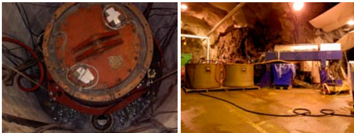
Figure 17-1. Demonstration of freeing of a copper canister by means of the hydrodynamic method in the Äspö HRL. The slurring of the bentonite buffer is shown at the left and the equipment for dewatering at the right.
