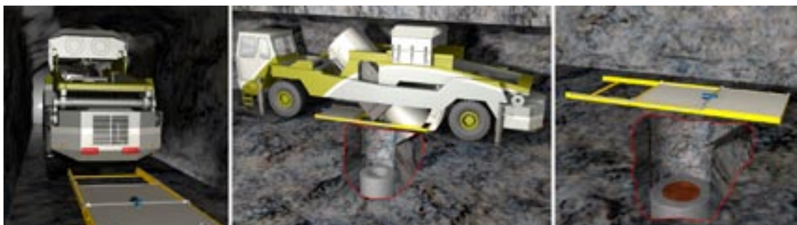
Figure 13-3. Radiation shielding hatch that prevents direct radiation before the uppermost bentonite blocks are put in place. The figure shows the radiation shielding hatch before, during and after deposition.
