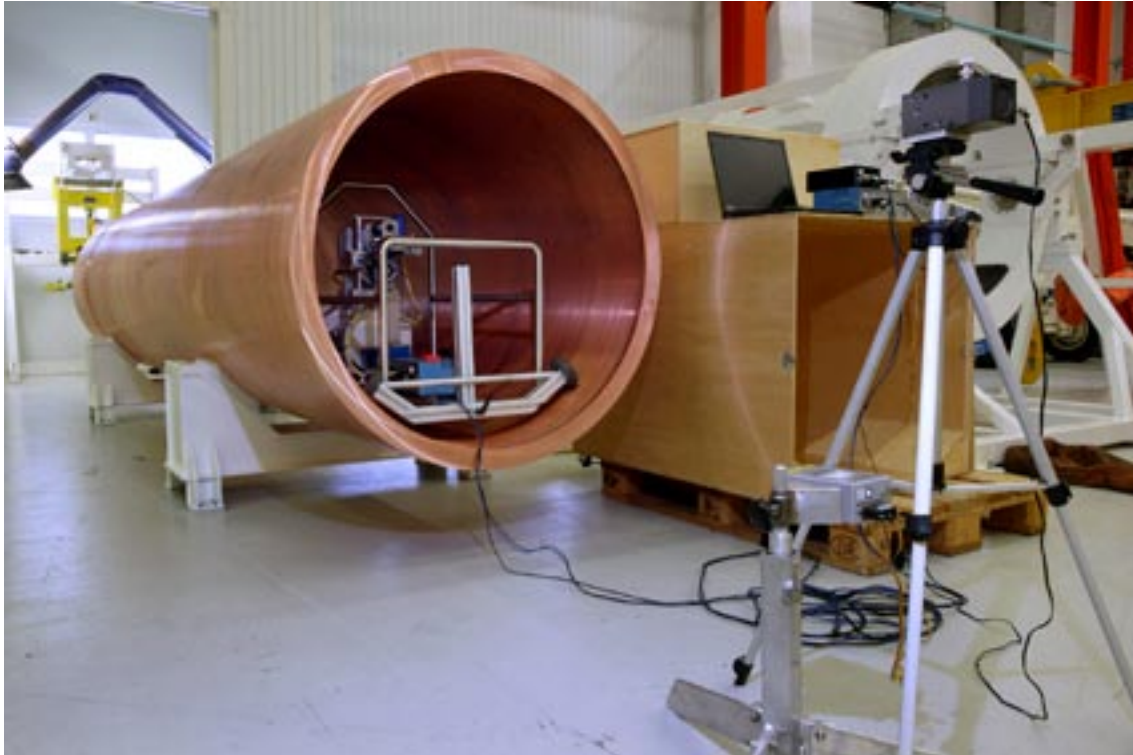
Figure 14-6. Laser measurement apparatus at the Canister Laboratory, December 2006.
