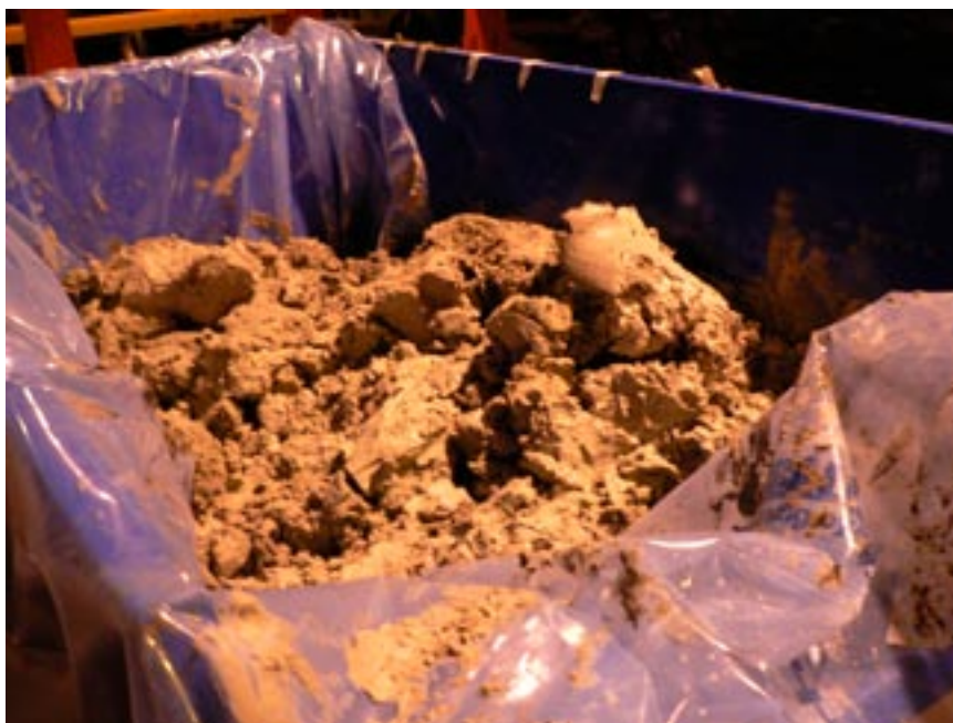
Figure 17-3. Dewatered bentonite from the decanter centrifuge.
