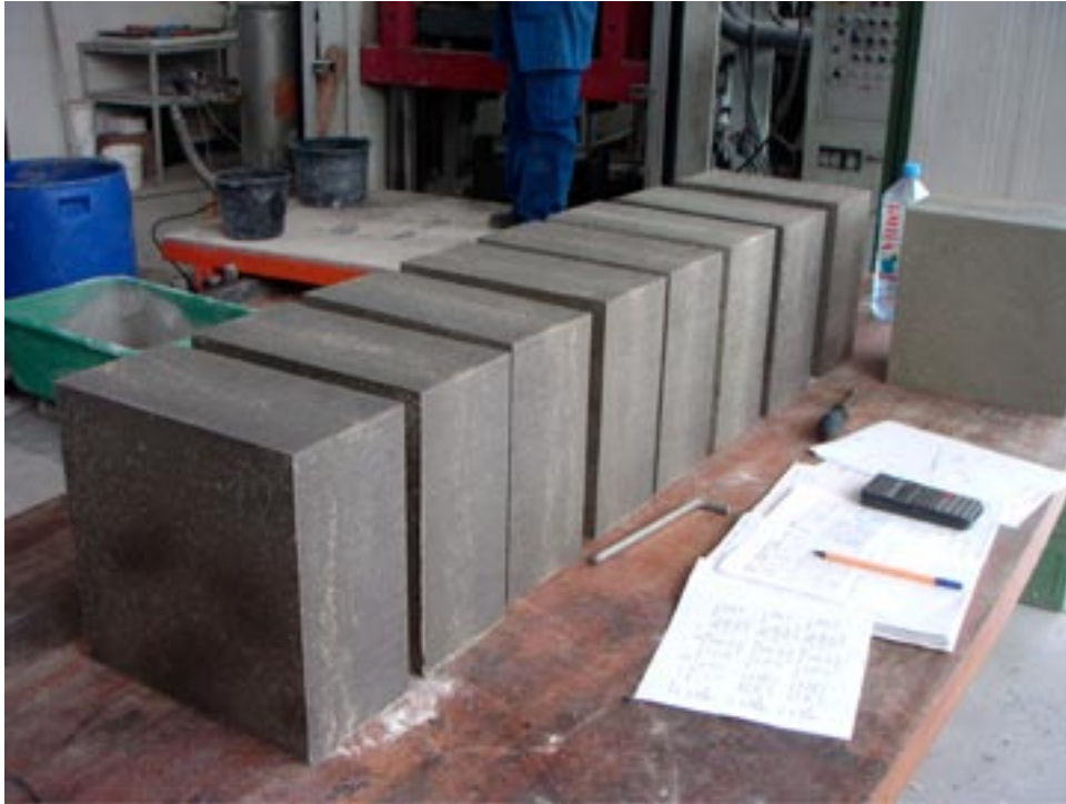
Figure 15-2. Some of the manufactured backfill blocks (300×300×160 millimetres).
