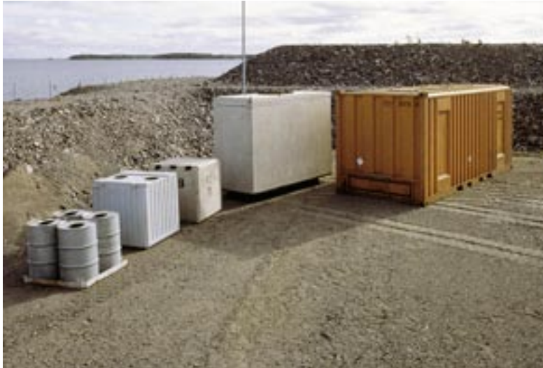
Figure 35-1. Waste containers for short-lived waste. Photo: Bengt O Nordin.
