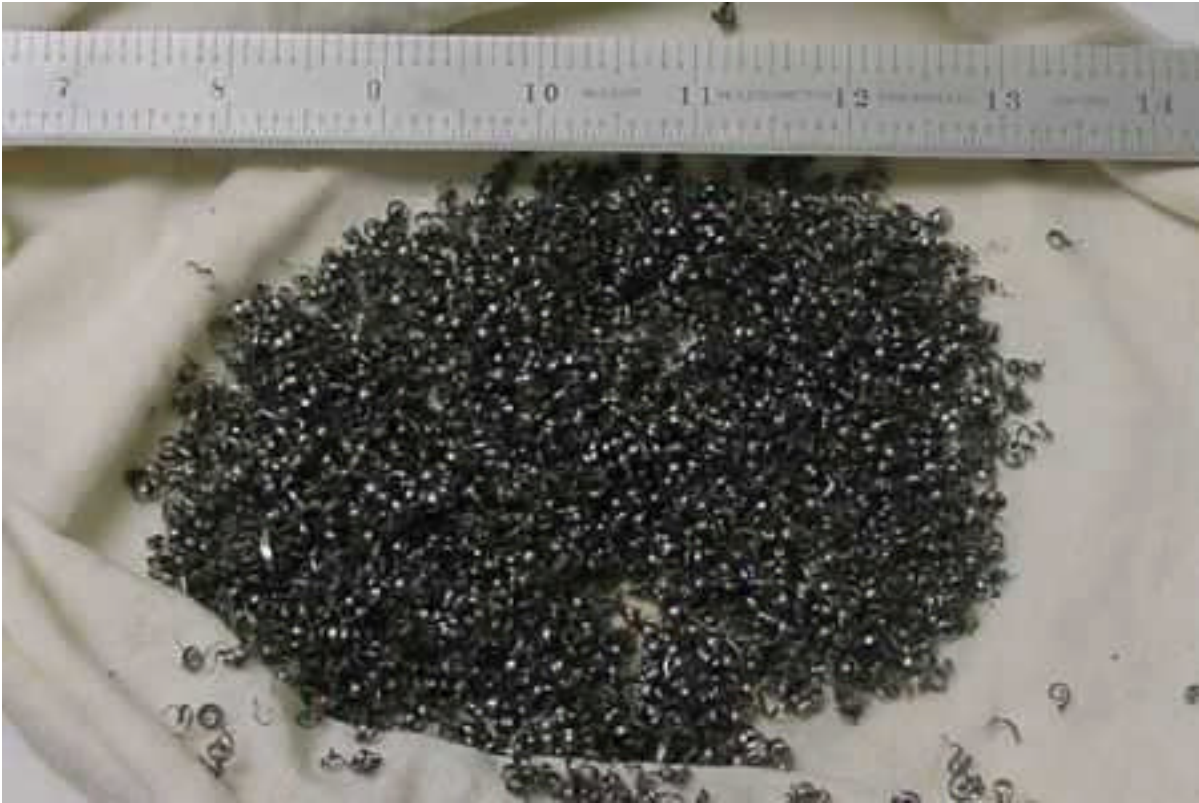
Figure 2 – Chips Created During Test Drilling in a Mockup Unit
