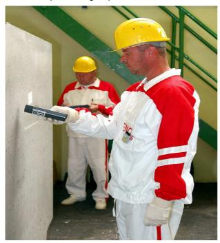
Fig. Monitoring of radioactivity on the surface of fibre-concrete containers
