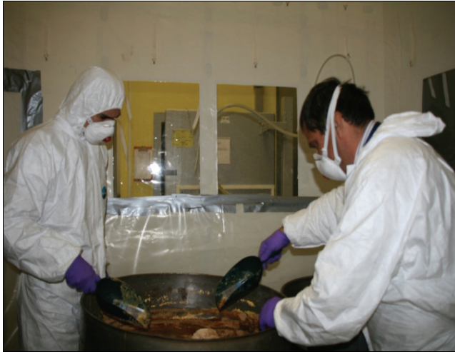
Figure 10: Filtration of spent ion exchange resins
