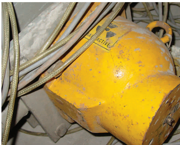
Figure 4: Disused sealed source Cs-137
