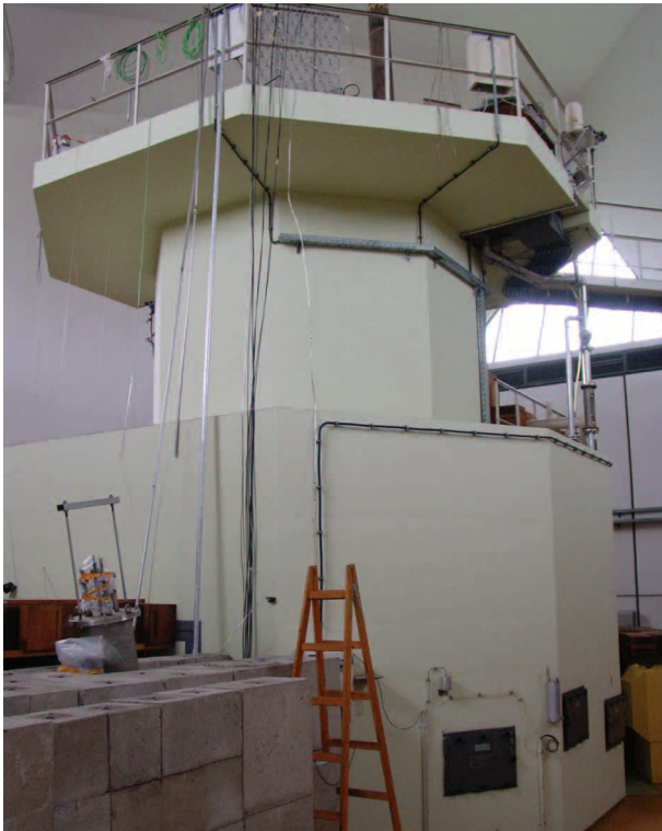
Figures 12 and 13: The reactor body and the reactor tank of the TRIGA Mark II research reactor
