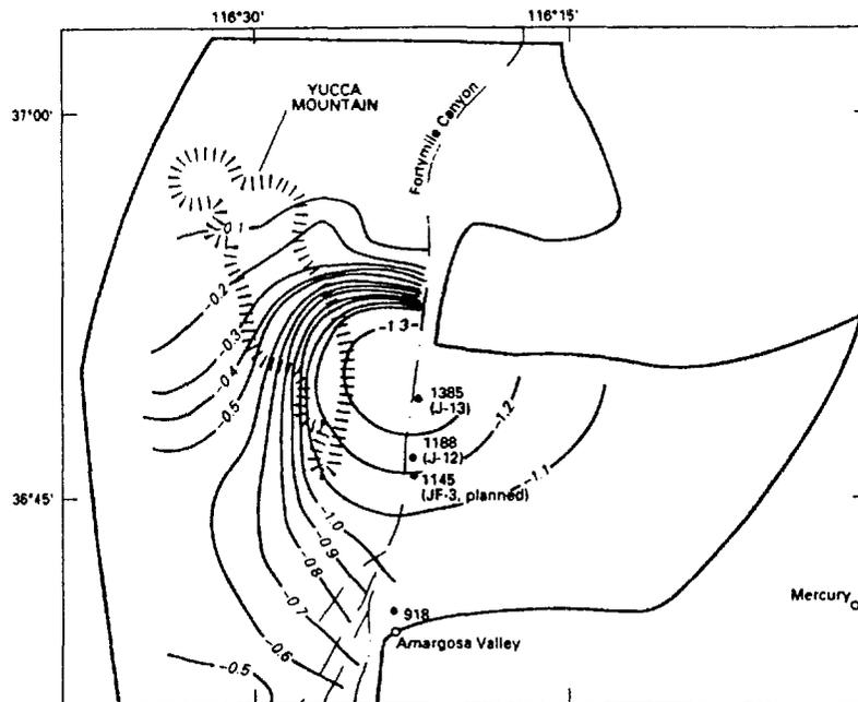
(a) Simulated water-level decline caused by well J-13 pumped at 138 gal/min and well J-12 pumped at 39 gal/min for 10 years.
