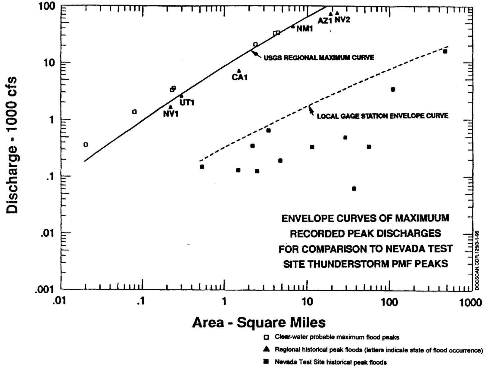
Figure 2.6.3-1 Envelope Curves - Maximum Peak Discharges (modified from Bullard, 1991)
