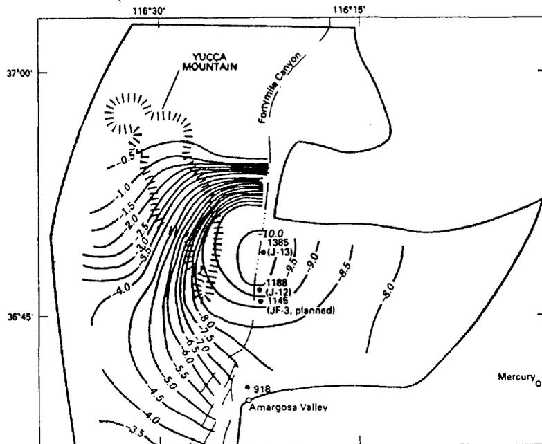
(b) Simulated water-level decline caused by well J-13 pumped at 630 gal/min and well J-12 pumped at 760 gal/min for 10 years.
