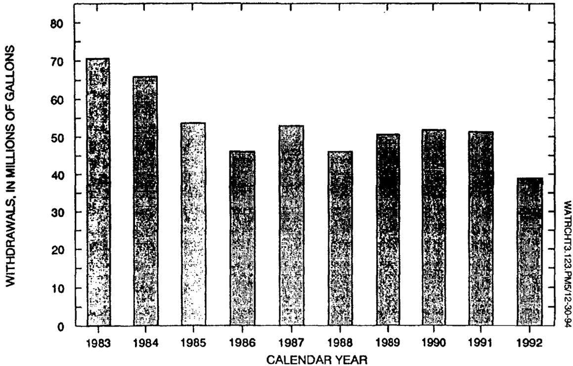
Figure 3.3-3 Water-level altitudes in wells J-13, J-12, and JF-3 and estimated ground-water withdrawals from Jackass Flats, 1983 through 1992. Bar height equals sum of withdrawals from water-supply wells J-13 and J-12. (from La Camera and Westenburg, 1994)
