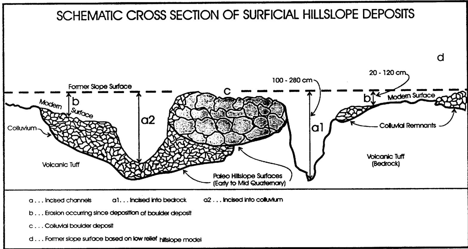
Figure 4.3.2.1-2 Schematic Cross Section of Surficial Hillslope Deposits
