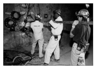
FIGURE 4 Photograph showing the 6-yard long, 4-kilowatt heater used in the single heater test in Alcove 5.
