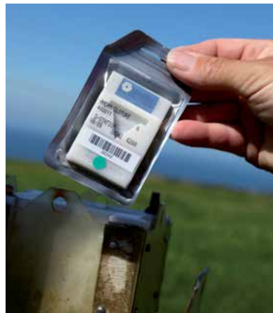
Dosimeter used to measure radioactivity around disposal facilities.
