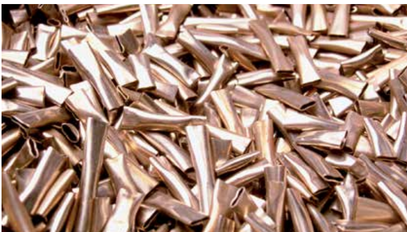
Waste metal from the structures surrounding spent fuel (hulls and end caps) that makes up ILW-LL.
