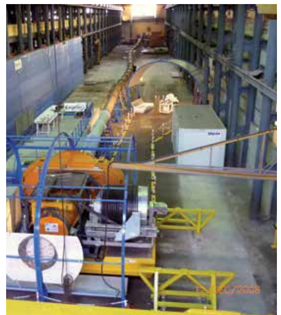
Test to retrieve a high-level waste package in a highly deformed disposal cell.
