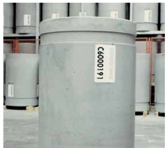
Concrete package of HLW (Height: 1.5 m, dia: 1 cm, approx. weight: 2 tonnes).
