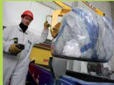
Compacted VLLW packages
