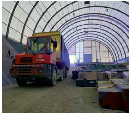
Disposal of a VLLW package in a cell at Cires
