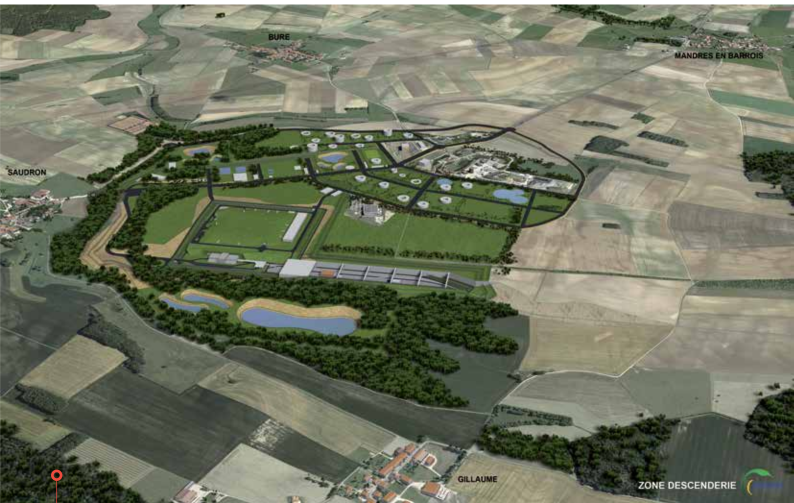
General view of the surface zone set aside for the receipt, inspection and preparation of waste packages - General layout including assumption of an on-site railhead.
