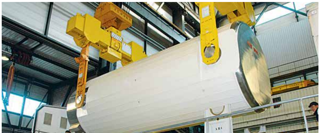
Transport cask in which HLW packages will be placed for transport. Each cask will be inspected prior to shipment.
