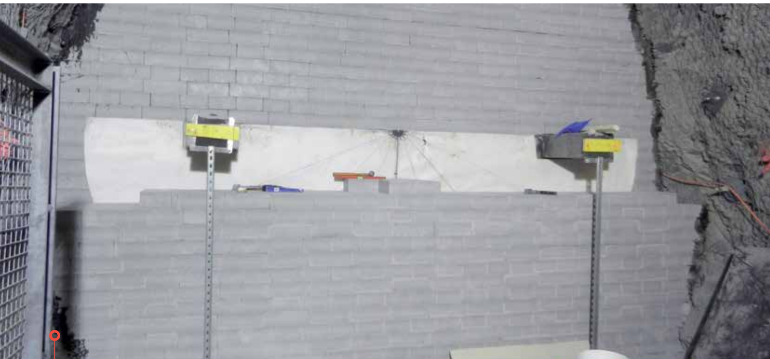
Sealing experiment in an underground laboratory drift.
