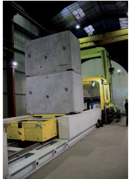
Test for emplacement and retrieval of ILW-LL waste packages
