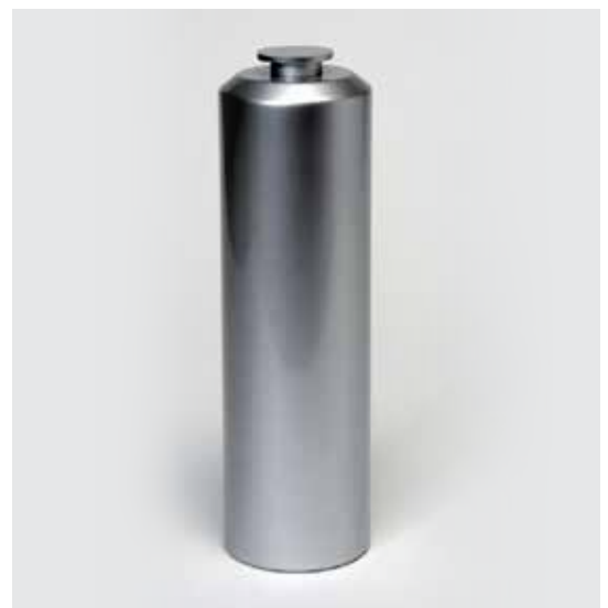
Package of vitrified HLW (Height: 1.3 m, dia: 43 cm, approx. weight: 500 kg).
