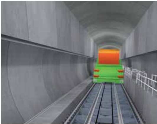
Transfer via funicular inside a ramp.
