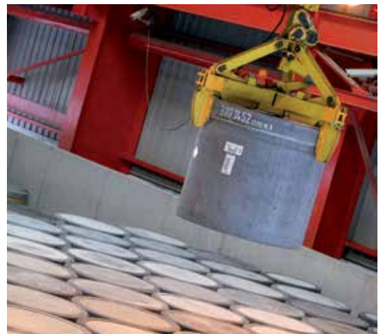
Disposal of a waste package in a CSA cell
