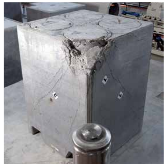
HLW-LL container demonstrator after a drop test.
